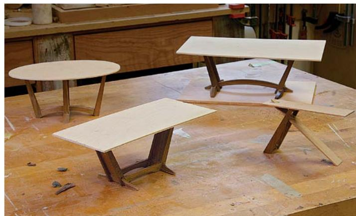
**Common scale.** Blaney builds  $\frac{1}{8}$ -scale models to see his emerging designs in three dimensions. Using solid wood and working fairly quickly, he joins them with hot glue and leaves out fine detail.
