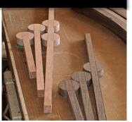
The curved elements are bent laminations made with ¼-in.-thick solid-wood plies clamped on a particleboard form. The lollipopshaped elements are laid out on a plank and bandsawn to shape.
