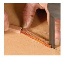
Make the convex cut. Once the posts have been fitted to the bar, saw the top edge of the bar to its convex shape. A piece of 1/4-in. MDF creates a zero-clearance table surface.
