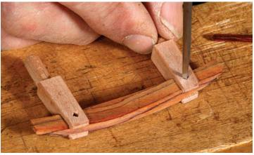
Follow with the chisel. Use a ½-in. chisel to chop the miniature mortises. To remove waste during chiseling, Day redrills with the ½-in. bit.
