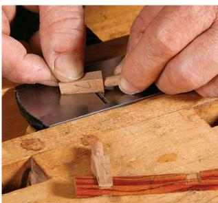
Slot for the bar. After crosscutting the ends of the workpiece at an 85° angle, use an angled guide block to cut the slot. Then cut a post blank from each end of the workpiece and repeat the process.
