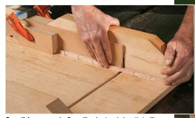
One stick, many posts. Day mills a long workpiece that will yield a batch of posts. He roughs out the tenons on the posts by dadoing across all four sides.
