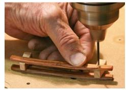
**Drill straight through.** With the pull dry-fitted and with a sacrificial table to back up the cut, drill right through both bars and the post with a ½-in.-dia. bit.
