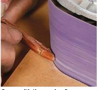
Scoop with the sander. Day uses his belt sander, clamped on its side and fitted with a shopmade "table," to shape the scooped sections at both ends of the bar.
