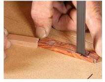
**Tiny dadoes.** With the bar blanks still milled square, use a crosscut sled with a stop block to cut the pairs of dadoes at both ends (left). Use a chisel to chop the outside shoulder of the dado to match the taper of the post (above left). Then carefully bandsaw the inner curve (above right), and fair the curve with files and sandpaper.
