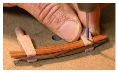
**Drilling for diamonds.** Before chiseling out the diamond-shaped mortise for the plug, drill a  $\frac{1}{10}$ -in.-dia. hole through the post and into the bar.
