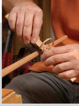
Bevel-up shaves are the traditional choice for shaping green Windsor chair spindles, because the low cutting angle follows the grain nicely. They handle end grain
