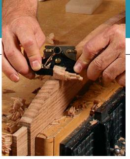
Start high and work low. Gochnour starts in the center and pushes toward the low end of the curve (left). To smooth the other side of the curve, he reverses his grip and pulls the shave, always cutting with the grain (below).
