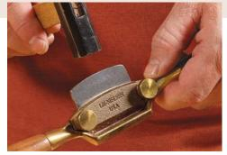
**Then tap it out.** A few taps with a small hammer on the back of the blade gets it into position. For lateral adjustments, tap on the side of the blade.
