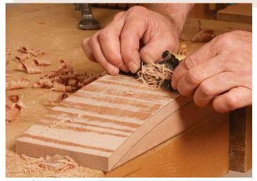
**Work wide curves evenly.** Gochnour works systematically to create an even surface on this drawer front—watching the bandsaw lines to keep him on track. This works well on narrow edges, too.
