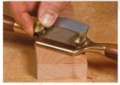
**Use a piece of wood to set it up.** Place the shave on a block of wood, insert the blade until it touches the wood, then tighten the screws.
