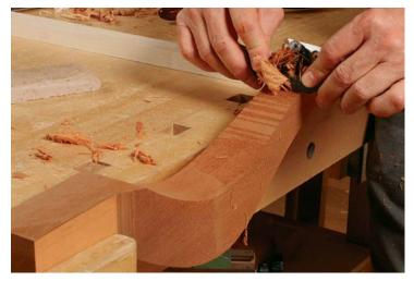
with 22.5° cuts. Finally, reset the blade for a light cut to make it even smoother. You can leave the last small facets if you like, or sand the profile smooth.
