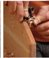
**Bullnose starts with a bevel.** Use a combination square to mark guide lines for the profile (above left). Shave to the lines to create 45° bevels, then do it again to create 22.5° corners. Set the shave for a lighter cut, and smooth away the remaining facets (right).
