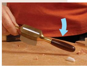
**Back out the blade for fine cuts.** The easiest way to do this is to flip over the spokeshave and tap it against the bench.
