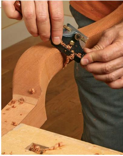
**Shape a curvy cabriole leg.** First Gochnour removes the sawmarks and smooths the curves (above left). With the overall shape established, he moves on to rounding and shaping the corners (above).
