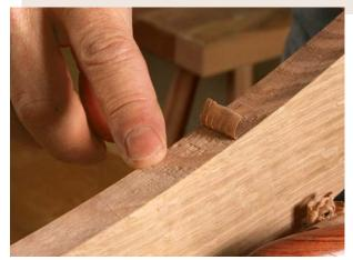
**Watch out for reversing grain.** If you notice tearout or feel the blade digging in, try cutting from the other direction. This tearout (above) is from cutting uphill in white oak. The best way to check for bumps and tearout is to run your fingers down the edge (right). They'll feel bumps you can't see.
