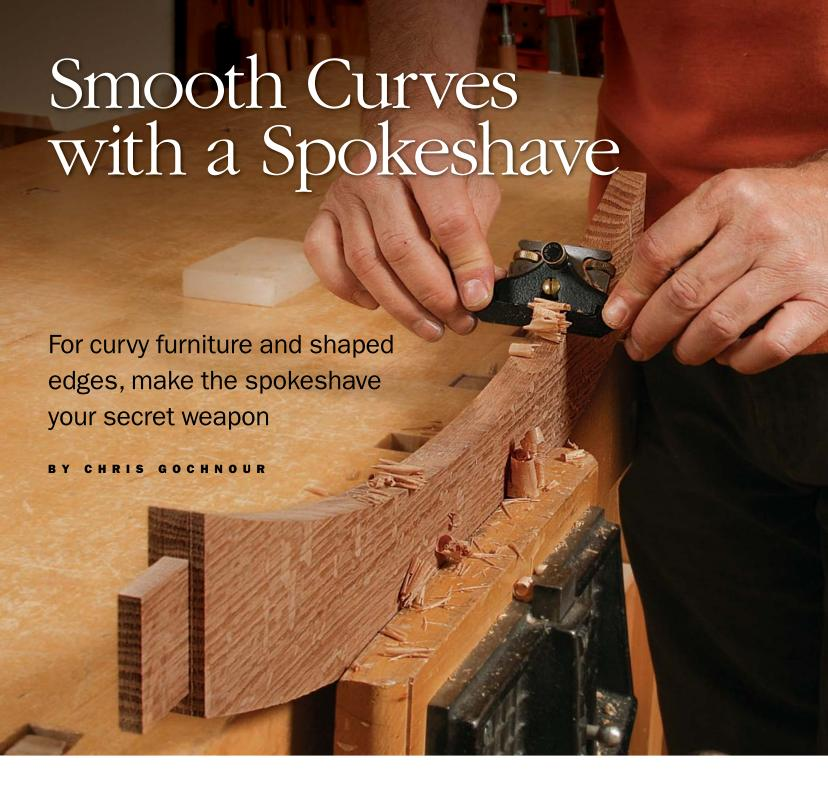
hen it comes to refining curves and shaping contoured work, there's nothing better than a spokeshave. Mechanically, a spokeshave works the same way as a handplane, but its small sole makes it ideally suited for following curves. After you've cut out your work on the bandsaw or router, a spokeshave steps in to remove sawmarks and irregularities with precise fingertip control.
