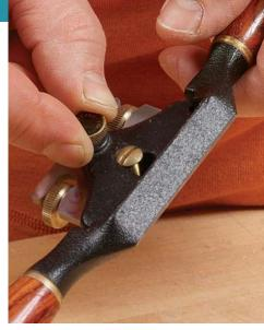
**Insert the blade and put on the cap.** Make sure the bevel is oriented correctly (down, in this case) and that it rests flat against the bed. Slip the cap iron into place and tighten the cap screw—enough to hold the blade securely, but still allow you to adjust it.
