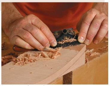
**Skew the shave for an easier start.** When it's tough to get the shave started, try holding it diagonally to the work. It makes the sole longer, so it's easier to smooth out those first few high spots.
