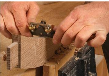
**Grip it and rip it.** Use your thumbs to push the shave (top), gripping both handles between your thumb and index fingers, and wrapping your other fingers around the handles. For a pull cut (bottom), turn the shave around and hold it the same way, but pull with your index fingers.
