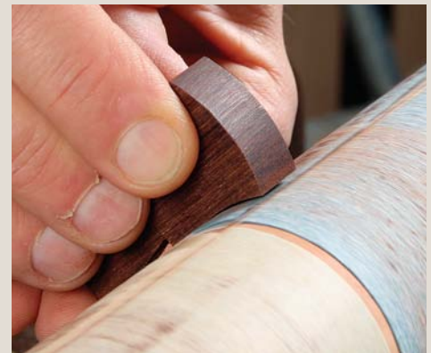
Clean up with a sander. After removing most of the waste at the bandsaw, Rousseau finishes shaping and smoothing at his shopmade spindle sander, which spins on his lathe.
