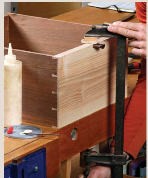
Clamp down. To prevent damage to the pull or drawer front, use a caul above the pull, and clamp to the bottom of the bench.
