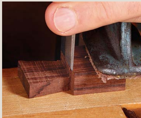
Clean up. After removing the tail and rabbet waste, pare down to the shoulder line.
