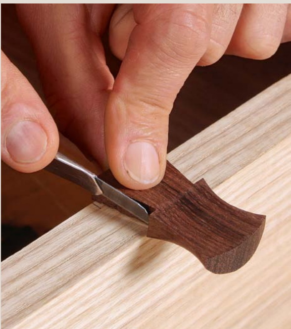
Cut the tail. After laying out the pull on a blank, Rousseau uses a jig sloped the same angle as the tail to cut the sloped sides. Begin the rabbet under the dovetail at the bandsaw, too.
