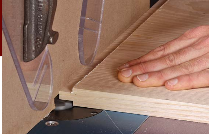
Two rabbets make a tenon. Rousseau cuts to the final depth and width on each side in a single pass.
