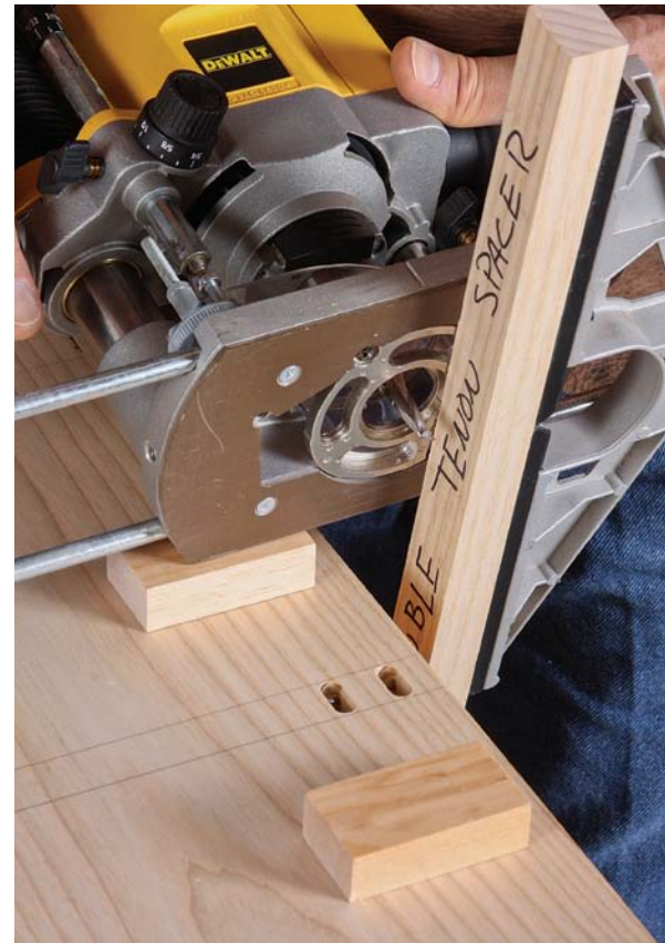
Add a spacer for the second mortise. The spacer's thickness equals the distance between the two mortises plus the bit's diameter. Attach it with double-sided tape.
