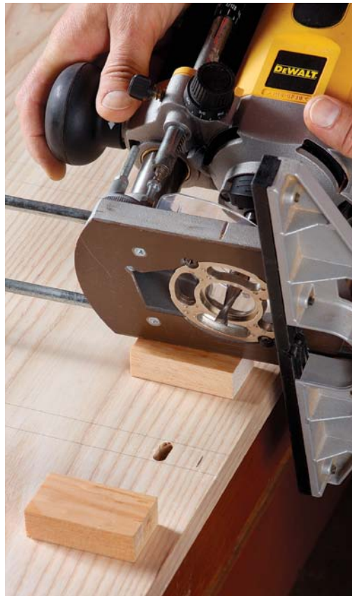
Inside mortise first. Set the edge guide (no spacer yet) so that the bit is located to rout the mortise farther from the edge.
