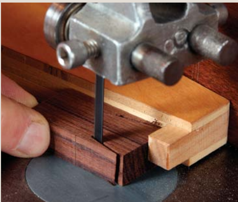
Cut the tail. After laying out the pull on a blank, Rousseau uses a jig sloped the same angle as the tail to cut the sloped sides. Begin the rabbet under the dovetail at the bandsaw, too.
