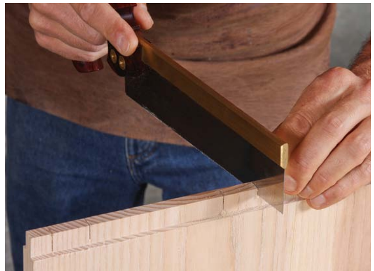
Saw down to the haunch. Use a backsaw to define the tenons, then cut the haunch at the bandsaw.
