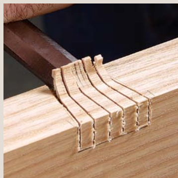
Lay out for the socket. In addition to transferring the tail's sides (left), also mark the socket's depth to match the tail's thickness. Remove the waste (above). Kerfing the waste between the cuts that define the socket's walls makes it much easier to chop out the waste. To avoid blowing out the corners on the narrow side, work toward the wider side of the socket.
