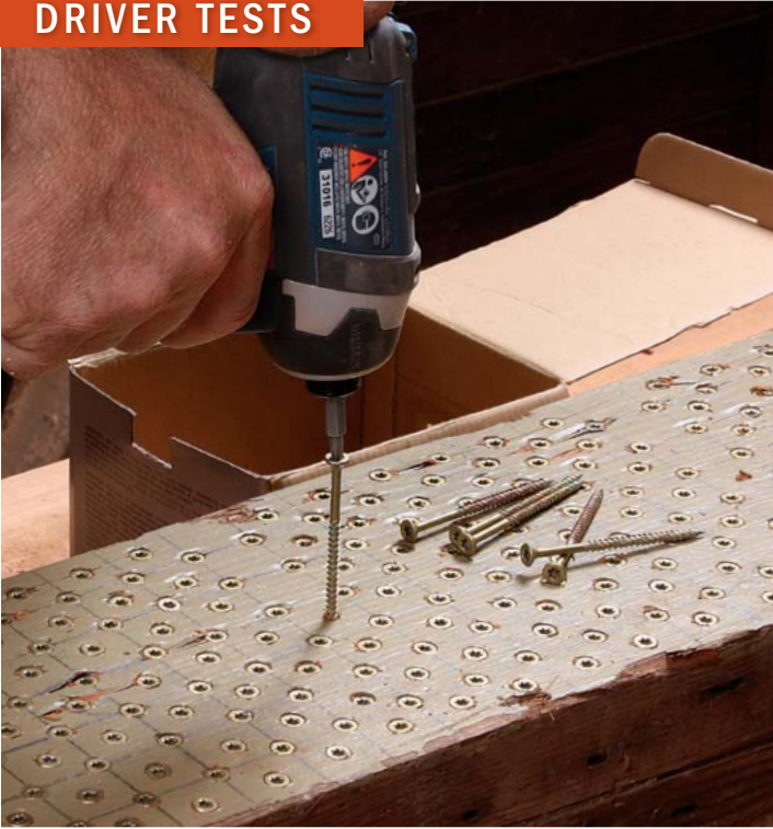
How many screws? Working with another section of that hard fir beam, Camp drove as many 3-in.-long screws as he could, with no pilot hole.
