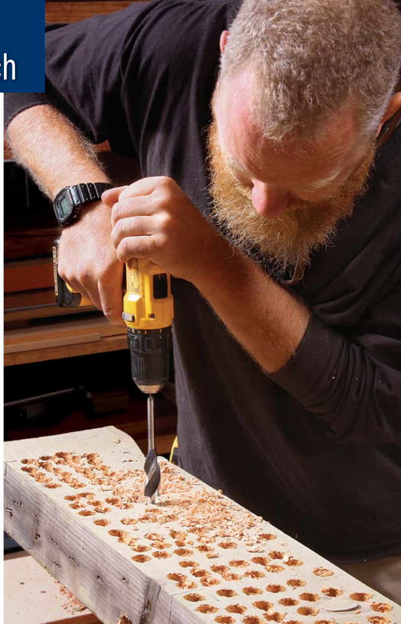
Even bigger bit. Using a \frac{3}{4} -in. Irwin Speedbor bit, Camp bored as many holes as he could through a 5\frac{1}{2} -in.-thick, old-growth fir beam. The DeWalt did well here.
