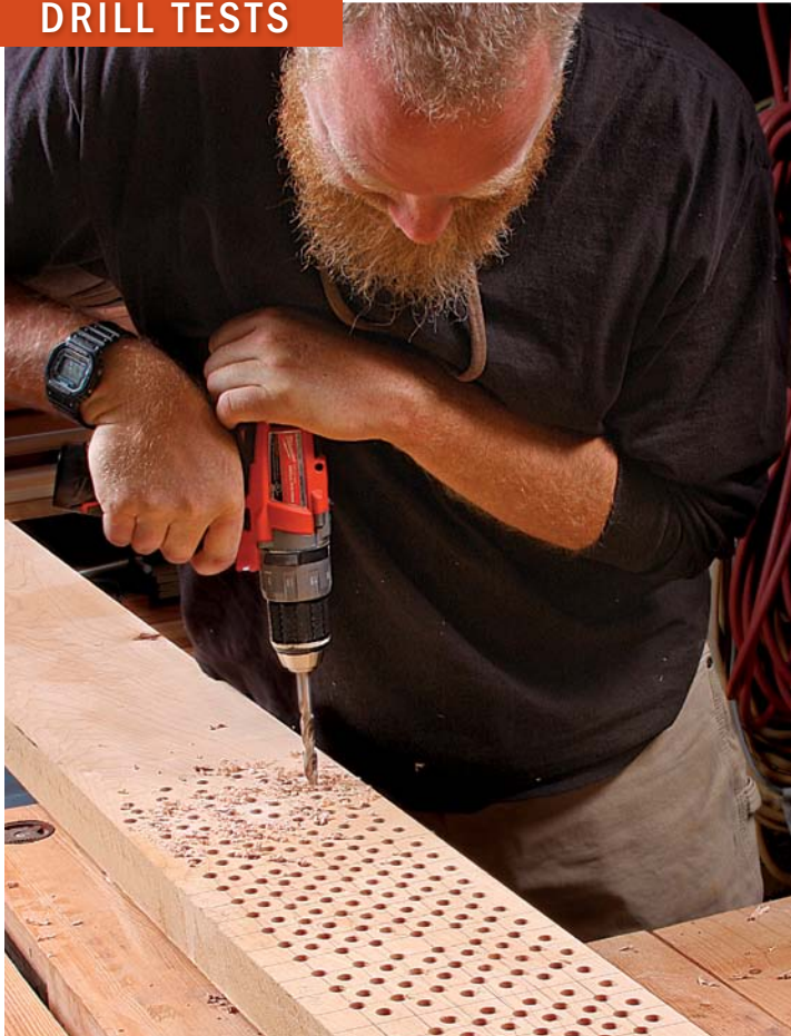
How many holes? Using a \frac{3}{8} -in. brad-point bit in hard maple, Camp drilled as many holes as he could on a single charge. Milwaukee's Fuel drill did almost four times as many as its competitors.
