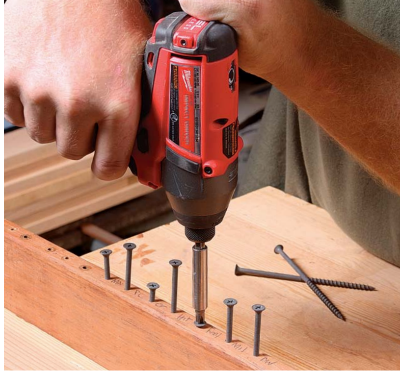
One for fun. To find the top-end torque of the drivers, Camp attempted to drive 4-in.-long screws into a very dense tropical hardwood, with an undersize pilot hole.
