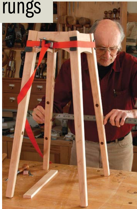
Reality check. Dry-assemble the legs and aprons and measure the length for each rung separately. Add 3/4 in. to each end for the tenons.
