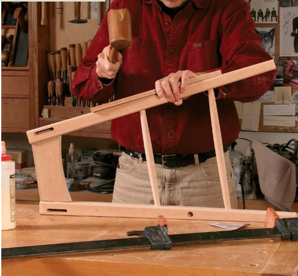
First the front and back. Glue up the front and back as separate units and set them aside to cure.
