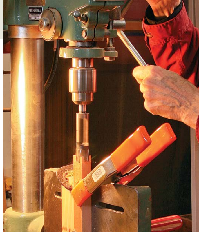
Tenoning rig. With the rung blanks milled square and cut to length, Becksvoort uses a tenon cutter in the drill press to cut the tenons on each end. Alternately, you can turn the tenons.
