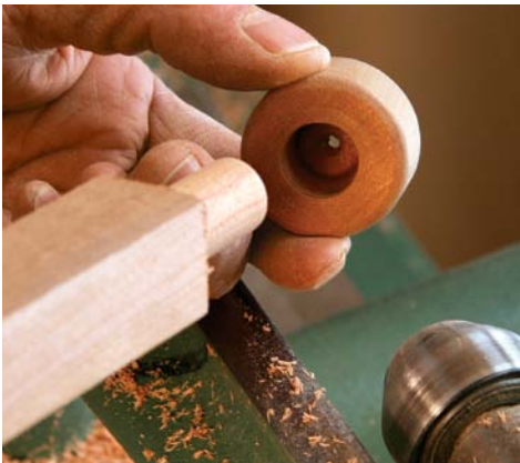
Clever doughnut. A scrap with a 5/8-in.-dia. recess drilled into it helps mount the rung on the lathe. The small, through centerhole seats on the lathe's dead center.
