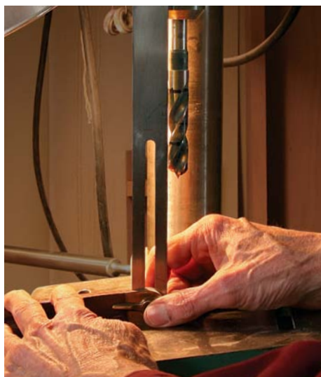
Taper two sides. Using a shopmade tapering jig, Becksvoort tapers the two inside faces of each leg. Then he cuts the mortises and rounds over the long edges of the leg on the router table.
