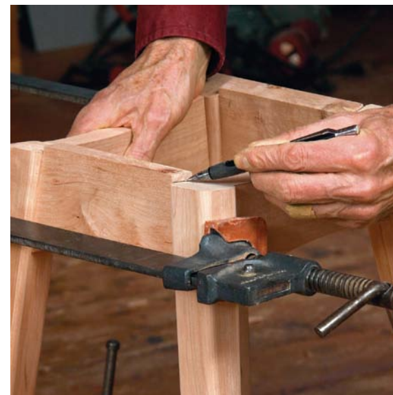
Dry-fit and draw a line. With the side rails and rungs dry-assembled, mark the side rails where they protrude above the leg. Then disassemble and trim to the line at the bandsaw or tablesaw.
