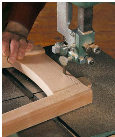
The top edge must mirror the seat. Trace the curve of the seat onto the legs and seat rail of the front and back units (left). With the subassembly riding inside face down, and the bandsaw table tilted 5\frac{1}{2}^\circ , cut along the curved line for the scooped seat (above).
