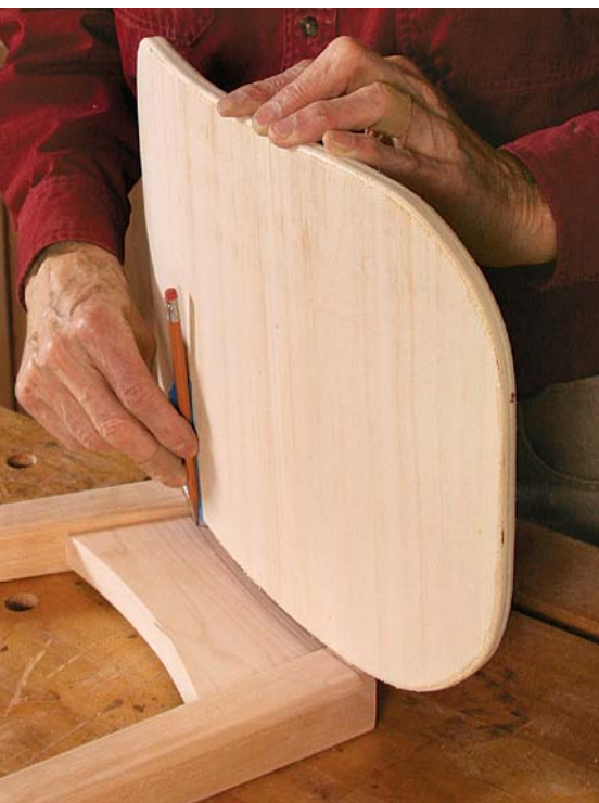
First the front and back. Glue up the front and back as separate units and set them aside to cure.
