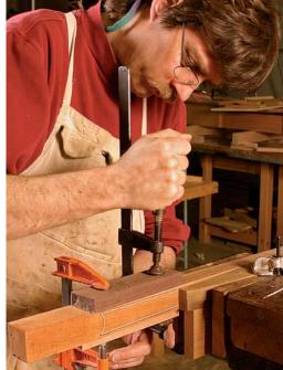
Glue in the pieces. Start with the outer pairs of petals, using a clamping caul lined with clear tape to prevent sticking. The next day, you can inlay the center petals.
