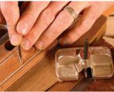
Excavate the recesses. Latta uses a Dremel tool fitted with a router base and a small spiral bit to remove the bulk of the wood (top). He cleans up the cut with a narrow chisel (above) and a router plane fitted with a pointed blade.
