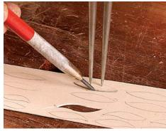
Lay out the petals. Cut out one petal of each size and use that as a template. The points of a divider work well to hold down the petal as you draw around it with a sharp pencil.
