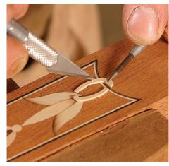
Delicate work. Make the loop that suspends the beliflowers from laminated holly veneer to prevent it from breaking. Inlay the two pieces in the same way as the petals.
