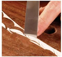
**Chop out the petals.** Use different-size carving gouges to slice out the petals from the holly veneer.
