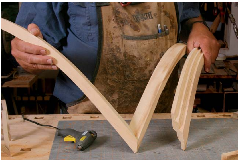
Full scale for detail. Rather than fussing with fine detail on a model, Fortune switched to a full-scale mock-up in pine to explore a stepped arrangement he had in mind for the table.
