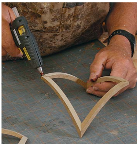
A little MDF goes a long way. Fortune cut short, curved pieces from a small scrap of \frac{1}{4} -in. MDF and hot-glued them together to make these models. He made extras and tried various groupings until he found the linked pairing he settled on.
