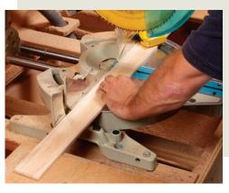
No mark needed on the miter saw. With the tape hooked on the end of the workpiece, just align the blade with your desired measurement. (without turning the saw on). Hold the workpiece tight against the fence.
