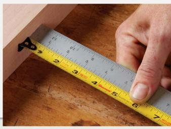
**Check the outside reading.** When you're in the store, grab a good steel ruler off the shelf, hook the tape on the end, and verify that the lines match.
