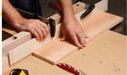
**Precise, matching parts.** A tape measure can do more than rough work. To cut two case sides the same length, for example, square one end of the workpiece, then hook your tape on that end and make a tick mark (left). Then use that tick mark to set up a stop (above)—in this case, a hook-shaped stop—and cut both parts precisely with one setup.
