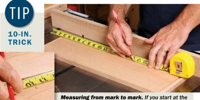
**Measuring from mark to mark.** If you start at the 1- or 2-in. mark when measuring from one pencil mark to another, you might forget to subtract that amount from your measurement. Start at 10 in. instead. That amount is hard to forget.
