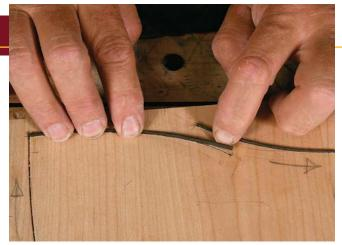
**Careful going cross-grain.** To avoid problems with wood movement, break up lines of inlay that run across the grain. Fortune limits cross-grain lines to  $3^{1/2}$  in. long, and he adds accent details between them.
