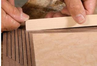
The inlay strip should press into the slit snugly with thumb pressure. After thicknessing and fitting the wide strips (left), Fortune bandsaws them to about 1/4 in. wide for inlaying.
