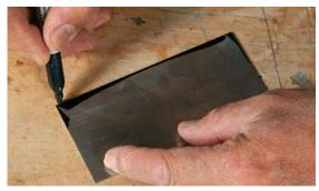
**Trace the profile.** Fortune marks the metal that he will grind away to create the tool's cutting teeth.
