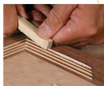
**Miters first.** Fortune inserts the mitered end of the strip first, then toes in the far end and finishes by pressing down in the middle (left). He uses the end of a small stick of soft pine as a push stick to be sure all the strips are well seated (above).
