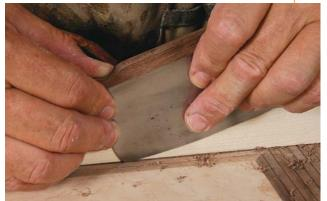
**Score, then go deep.** Several light passes with the curved tooth along the length of the layout line (left) score the edges. Fortune starts and stops just shy of the ends. A few heavier passes (above) get him to full depth. Before cutting the grooves, he lightly coats the wood with silicone-free wax so it will resist the glue.
