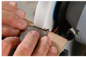
**Grind your teeth.** Making short, light passes against a grinding wheel to avoid heat buildup, Fortune removes the marked section of the scraper.
