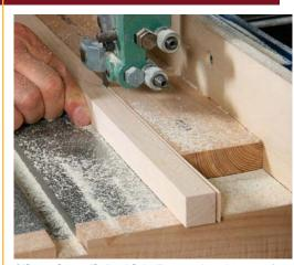
**Slice mine a little thick.** Fortune bandsaws strips for the inlay from 1-in.-thick stock. He rips the strips just slightly over final thickness and joints the edge of the stock between rips.
