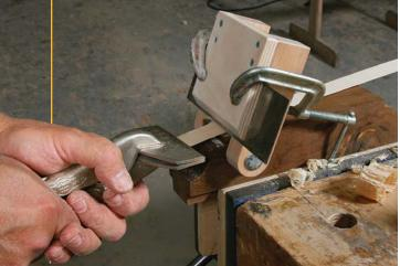
**Self-powered planer.** A few passes through Fortune's shopmade thickness scraper brings the wide strips down to final thickness—and cleans up the bandsawn face. Pull the strip through at a slight angle, so the bandsaw ridges don't catch. After taking a shaving, use the bandsaw marks as a guide to be sure the scraper is parallel to the jig body.
