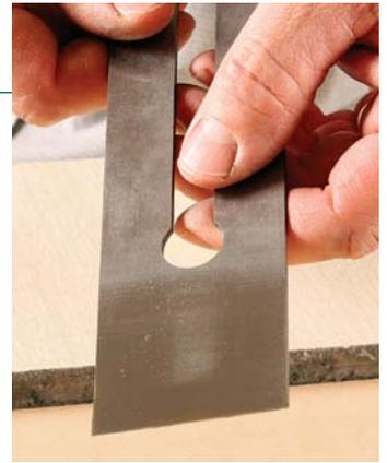
**Start with 150 grit.** Apply pressure with fingers from both hands within about  $\frac{1}{2}$  in. of the cutting edge (left) to ensure that the blade is flat on the sandpaper. Move the blade from side to side along the length of the paper, not in and out. Stay at this grit until there is a consistent scratch pattern extended back an inch or two from the cutting edge (above).
