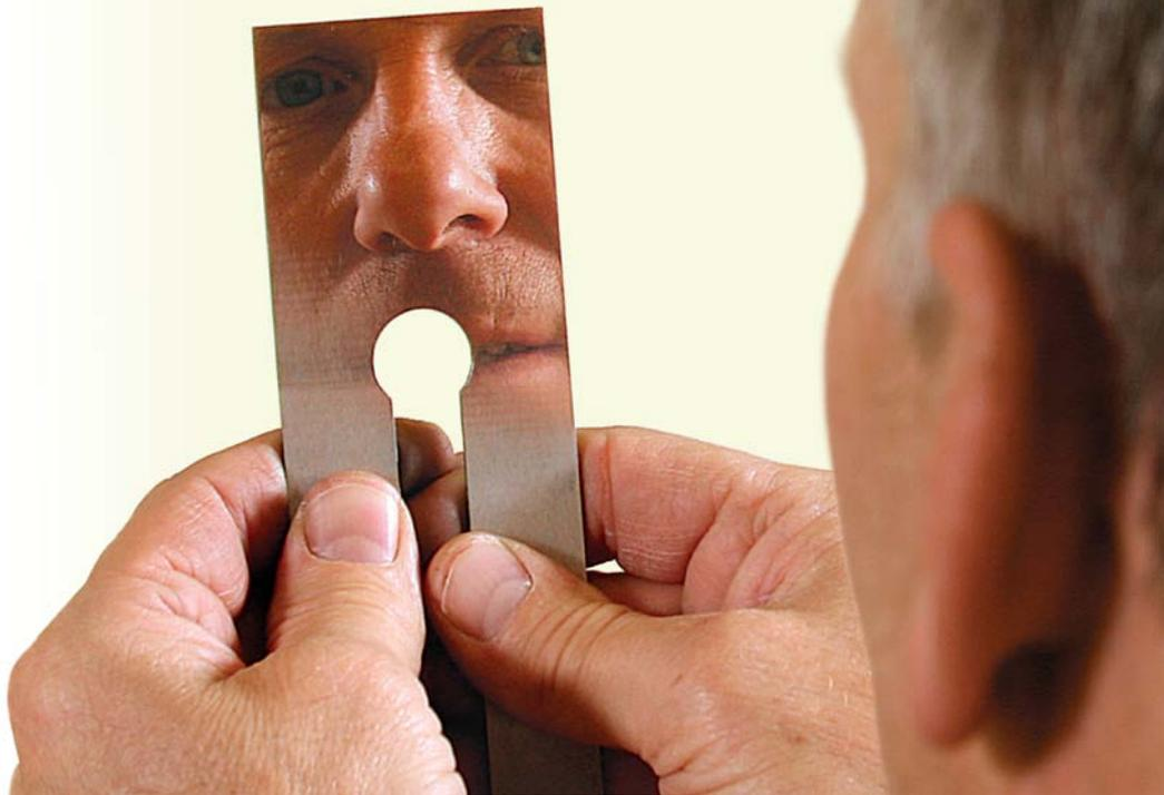
**Clear as a mirror, sharp as a razor.** The high polish means that the back—and the cutting edge—is truly flat and without blemishes. When it meets a bevel that's just as polished, the blade will be truly sharp.
