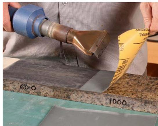
**Easy off.** To pull off the sandpaper cleanly, use a heat gun or hair dryer to soften the adhesive. Mineral spirits cleans up the leftover glue on the granite.
