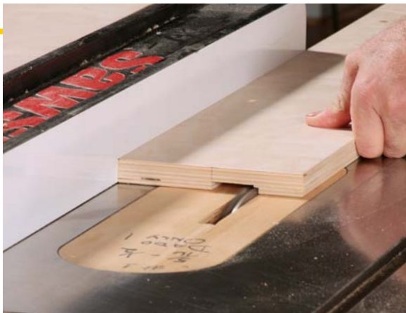
Wide grooves house the bridge. Use a \frac{3}{4} -in. dado cutter and make multiple passes to achieve the desired width.
