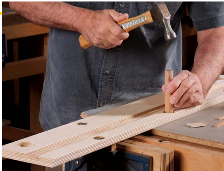
Install the hardware. Use a Forstner bit and a Brad-point bit at the drill press to drill a set of stepped holes. Epoxy a T-nut-style threaded insert into each hole. A dowel and hammer help seat each nut.
