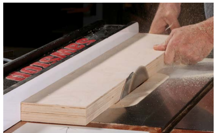
Trim to fit. Rip both edges of the bridge to ensure they are straight and parallel, and slightly wider than your rip fence.
