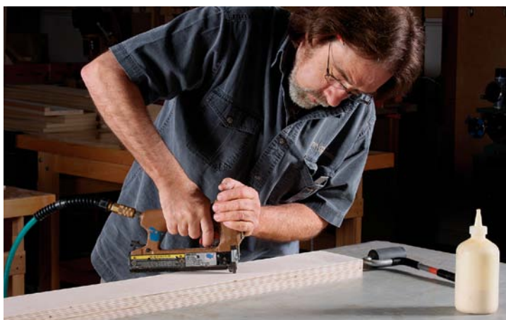
Glue up the bridge. The central piece of the base is made from two layers of plywood, glued and nailed together.
