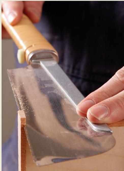
**Ride the spine.** As you saw, press down on the spine to keep the teeth away from the surface. Use a chisel or block plane to flush the edging.
