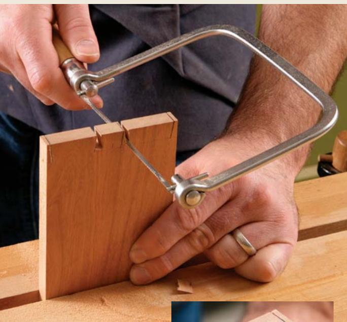
**The teeth face the handle.** This means the saw cuts on the pull stroke, which puts the thin, narrow blade under tension so it won't buckle.
