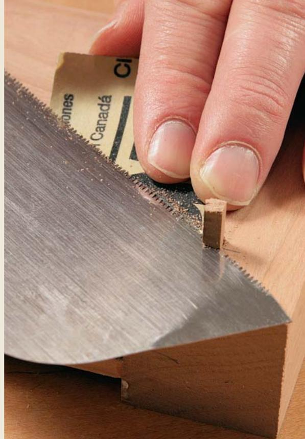
**Sandpaper prevents scratches.** Where the spine trick won't work, fold a small piece of sandpaper (abrasive side in) and put it under the blade to prevent the teeth from marring the wood.
