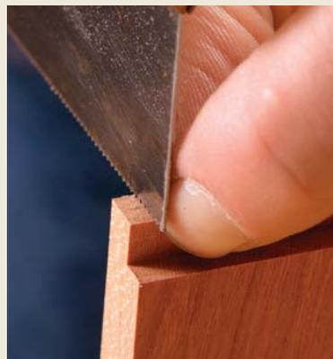
**Easy way to start the cut.** After cutting a line with a knife or marking gauge, put the nail of your forefinger and thumb into it, place the saw's teeth against the nails, and push lightly.
