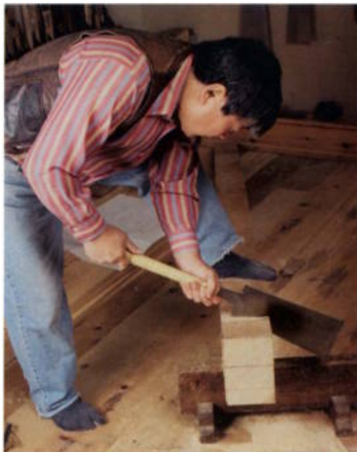
Using two hands on the ryoba-noko yields maximum power and control. Here the author cuts a tenon's shoulder, using the saw's crosscutting teeth. He'll flip the saw over and use the rip teeth on the other edge for cutting the tenon's cheeks.
