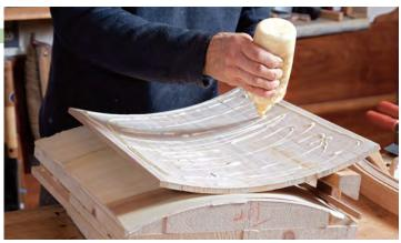
**Apply glue to core.** An even, generous layer of glue across the core helps create a solid joint without voids. Don't spread glue on the veneer, as moisture from the glue could ripple the stock.
