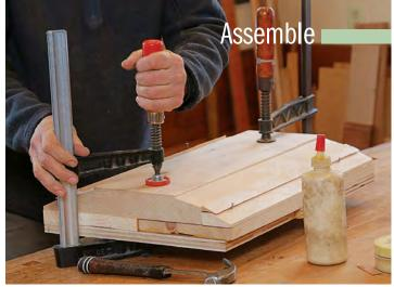
**Glue up the rough form.** Hack clamps where he can, but elsewhere simply nails down the beveled parts to keep them in place while the glue dries.
