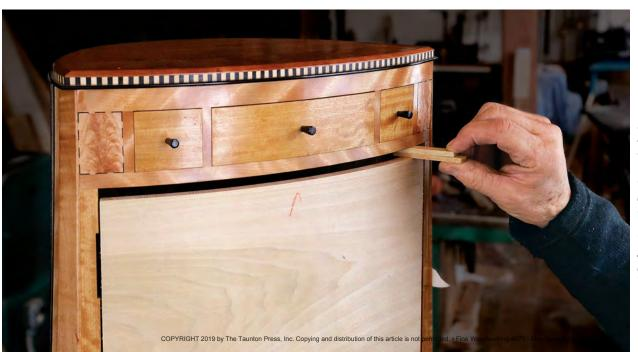
Door size should account for edge-banding. When setting the door gaps, use two pieces of edge-banding as shims. Trim the door until the spacing is what you want. At this point, tight is better than loose.
