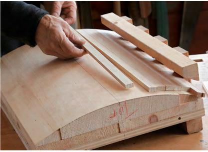
**Make the staves.** Hack tips the handplane (left) to form angled edges on each stave. These joints don't need to be perfect, so he finds the mating angles by trial and error, correcting each stave as he moves along. An extralong strip against the ladder will help distribute clamping pressure later.
