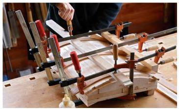
**Long, centered caul keeps the middle from lifting.** Hack calls this his strongback, and it's used to prevent the clamping pressure across the core from pinching the staves out of shape.
