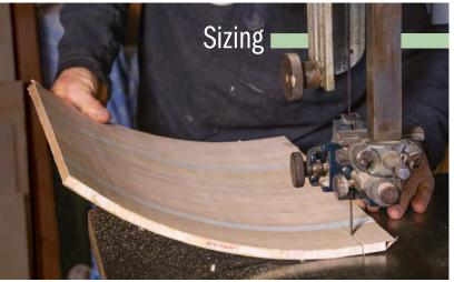
**Trim the core roughly to shape.** Hack uses a bandsaw and cuts close to his line. When sizing the core, be careful not to saw off the hardwood hinge-side stave.
