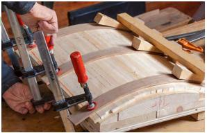
Bendable cauls distribute pressure. To get pressure across the face of the core, Hack first wedges ½-in.-thick, flexible oak cauls under the ladder. He then clamps down their loose ends. A wedge-shaped clamping block under the form prevents the clamps from slipping. An extra, unglued stave, marked with red, helps with the next step.
