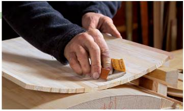
Fair the core's surfaces. To ensure a good mating surface for the crossgrain veneer, smooth both faces of the core. A plane works well for the convex face. For the concave face, Hack likes sandpaper backed with a thick piece of leather.
