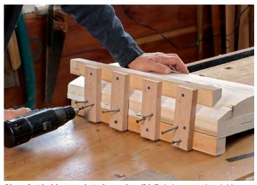
**Clamping ladder needs to be rock solid.** To help secure bendable cauls, Hack attaches a ladder of sorts to the side of the form. He uses plenty of screws, as it will be under lots of stress.
