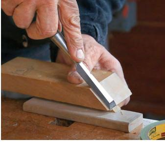
**Miters with paring block.** Hack miters the edge-banding for the door's two outside corners. On the hinge side, where the joint won't be seen, he uses a simple butt joint.
