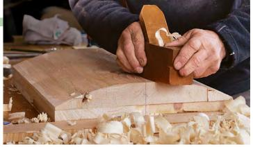
**Begin shaping the form.** Start with coarse cuts to bring the form nearly to shape, but don't hit your layout lines just yet.
