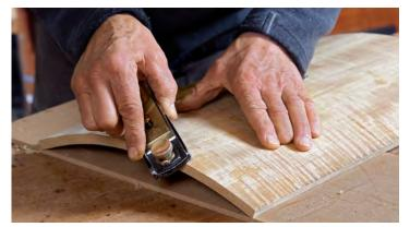
**Finish up the edge-banding.** Use a finely set plane to bring the face veneer flush with the edge-banding. Then, plane a chamfer the depth of the veneer. With a good color and grain match on the edging and face veneer, the joint disappears.
