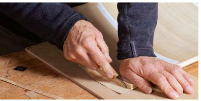
**End grain may need to be cut flush without spacer.** Veneer with wily grain may chip as it's cut to rough length. If this happens, forgo the spacer and take light cuts with the knife.
