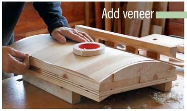
**Secure the cross-grain veneer to the form.** Tape down the veneer so it stays put when you glue it to the core. Keep the tape on the perimeter of the oversize sheet so it doesn't interfere with the joint.
