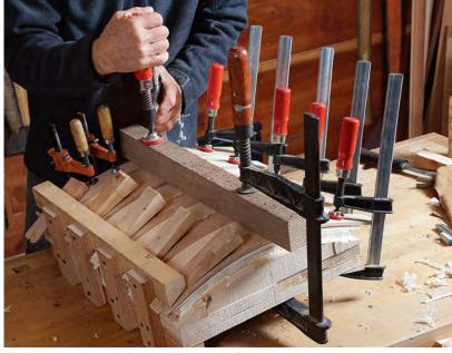
**Wedges, cauls, and clamps.** When clamping the cross-grain veneer, Hack uses three sheets of thin bendable plywood under the oak strips to distribute pressure. He also clamps the strips this time before wedging them so they don't shift the coopered core.
