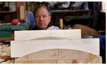
**Winding sticks check for twist.** To make the winding sticks, joint one edge of a pair of boards and cut the other edge to match the curve of the form. Sight across them to make sure the form is not twisted.
