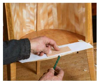
**Outside curve comes first.** Trace the exterior shape of the opening onto a piece of paper. Use a thin piece of scrap to back up the pencil and keep the paper flat. Cut out this arc with scissors.
