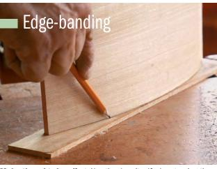
**Make the edge-banding.** Use the door itself when tracing the curved pieces. Cut them out overwide at the bandsaw. Rip the straight pieces, also overwide, for the side edges.
