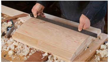
**Crayon and straightedge mark flatness along length.** Rubbing crayon on a straightedge and sliding it back and forth lets you know when the form's flat—a crucial step to ensuring a successful glue-up.
