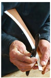
Make a hardwood template. After cutting out the paper template, glue it to a piece of hardwood and saw close to the line for the inner curve. Refine the curve with hand tools.
