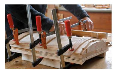
**Clamp across the door.** Apply just enough pressure to keep the joints closed without buckling them. For gentler curves, like the one here, a clamp works just fine. For tighter radii, wedges may be the way to go.
