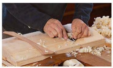
**Cross-grain cuts knock down ridges.** A nimble block plane used cross-grain lets you plane down localized areas easily. Keep the template on hand and check your progress often.
