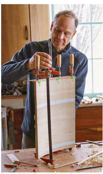
**Use tape and clamps for curved ends.** Hack relies on green tape because it's very elastic. To protect the edge-banding, he uses the hardwood template as a caul.
