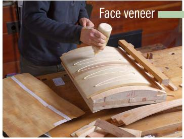
**Follow the same clamping steps.** After gluing and clamping the face veneer, make sure there's even squeeze-out along the seams. Adjust your clamping as necessary.
