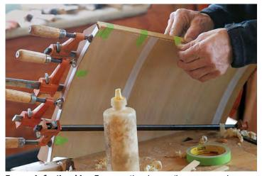
**Tape only for the sides.** To ensure there's enough pressure, make sure the tape's pulled taut across the joint. Flush up the edge-banding before adding the final layer of veneer.
