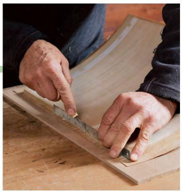
**After the glue-up, use a spacer when trimming the veneer.**Shimming out the knife lets you clean up the joint with a plane later.
