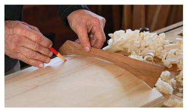
**Template and light reveal high spots early on.** Regularly hold the template to the form to see where you still need to plane down. Mark these high spots. Be sure to keep the template centered.
