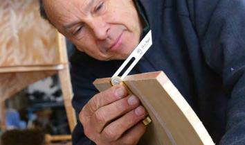
Bevel the edges of the side staves. Set a bevel gauge to the angle of the opening and plane the sides of the door to match. The hinge side should mate perfectly, but Hack slightly undercuts the other side so the door closes more easily.
