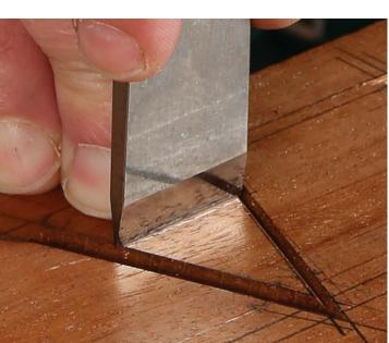
**Vertical strokes before horizontals.** Cuts parallel to the grain require stop cuts at the ends to prevent the grain from splitting. On letters like A, where the horizontal cut falls between two verticals, carving the verticals first creates natural stops for the horizontal stroke.
