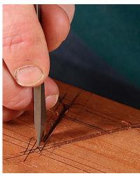
**Use a fishtail chisel to make a pair of stop cuts.** The stop cuts begin at the top center of the thicker trench, with one pointing up to the apex of the junction, and the other roughly perpendicular to the thinner stroke (left). Continue the center line of the stroke to the stop cuts (right).
