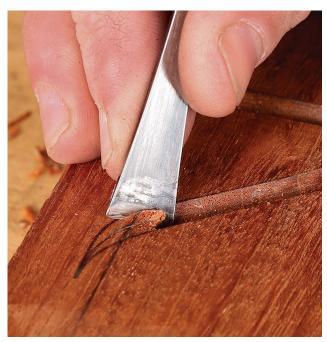
Continue with the curve. Use a gouge with a sweep that matches the curve to make a vertical cut along the centerline (far left). Then use a fishtail gouge to slice the curved walls (left).
