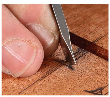
A pair of cuts at a serif. When a horizontal stoke ends at a serif such as the middle bar of an F, make a pair of cuts in a V-shape just before the serif to sever the end grain. Then carve the trench. Make the vertical and angled chops (below) and the chips should pop out cleanly.
