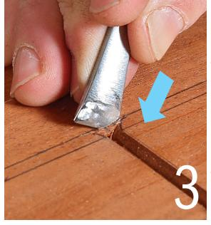
Finish with the end of the serif. Using a #3 fishtail gouge, start at one corner of the serif, angle it, and push down. You should end with the gouge's leading corner at the root of the serif, and its edge along the opposite corner of the serif. The gouge gives the serif its slightly incurved end wall.
