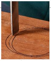
Make a vertical cut along the centerline. Work your way along the line with a gouge, fitting the shape of the gouge to the curve as you go.
