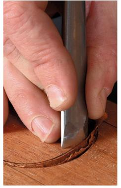
Pare to the line. With a sharp #4-16mm gouge, make a slicing cut all the way around the outside rim of the letter (above). Use a pencil grip and twist the gouge as needed to keep it on track. Keep the gouge tilted back toward you and remember to maintain the 30° angle. You may need to switch hands or body positions to work all the way around the letter. Finally, make a slicing pass on the inside trench wall, switching between a #3-12mm and a #4-12mm to adjust for the curve (left).
