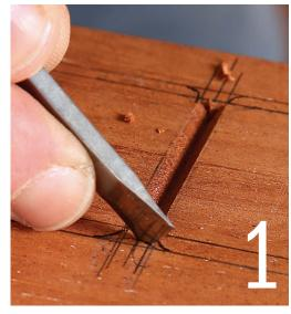
Make a pair of stop cuts. Start by planting the corner of the fishtail chisel at the centerline of the trench, then pressing forward at a 45° angle until the cut reaches the corner of the serif.
