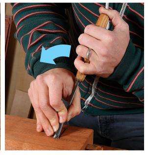
center line to the points of the serif. Then use a #5 fishtail gouge to cut the flaring side walls. The idea is for the letter to transition smoothly from a straight stroke to a curved serif. Next, cut the end of the serif using the #3 fishtail gouge, starting at the top of one corner and slicing down diagonally toward the other. If all has gone well, a little triangular chip should pop out, and the three faces of the serif should join in a point in the middle.
