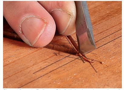
**Clear out the waste.** Finally, use a fishtail chisel to chop and remove the small chip left at the top of the larger trench.
