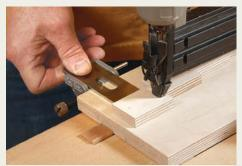
**Set your stops.** With the blade set at the desired angle, push the front of the guide flush with the edge of the jig base. Set the stop so it just touches the blade's edge, then nail it down.
