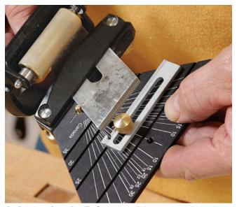
**Optional registration jig for skews.** This one has radiating lines to guide the skew angle, and a stop that lets you set the honing angle from 10° to 45° in 5° increments.
