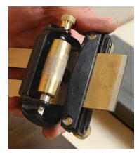
Do a barrel roll. The barrel-shaped roller lets you easily hone a camber, a slightly radiused edge, which is helpful for avoiding plane tracks.
