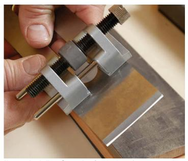
**Narrow wheel allows for camber.** Steady, alternating pressure at the corners of the iron produce a slightly radiused edge.
