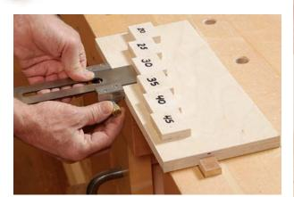
**Projection of blade determines honing angle.** Like other side-clamping guides, the Lie-Nielsen works best when paired with a shopmade projection guide for repeatable results.
