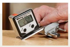
**Find the angle.** A digital angle finder is a simple way to find honing angles. Once the blade is at the angle, lock down the jaws.
