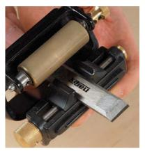
Switch to the side-clamping jaws for narrow blades and chisels. These jaws hold blades 1/8 in. to 11/2 in. wide and work with the square projection jig.
