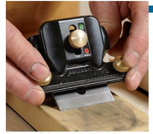
**On the stone is Gochnour's go-to.** While guides that ride on the stone typically restrict the amount of usable stone, they keep the honing angle constant from stone to stone regardless of differences in the stones' heights.
