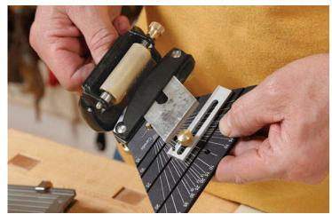
Top clamping is more versatile. Guides that hold blades from the top and bottom can secure them at a variety of angles in addition to holding them square—although positively and consistently registering these angles can be tricky. Gochnour has found that there's also a greater chance blades will slip out of their setting with these guides.
