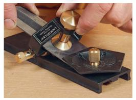
Angle guidance. The system includes an angle jig for setting bevel angles from 15° to 35°. It also has a cam for conveniently adjusting a microbevel.
