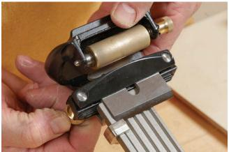
Guide for square blades included. The guide comes with a gauge for setting bevel angles from 15° to 54° and back bevels from 10° to 20°. Using it also helps set blades square.
