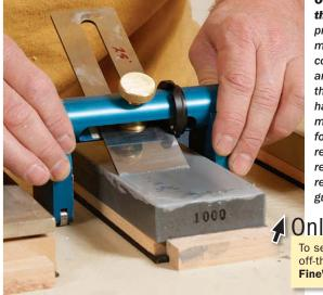
Off the stone is less than stellar. While they prevent the sharpening medium's grit from contaminating the wheels and let you use more of the stone, these guides have a catch: All stones must be the same height for the honing angle to remain constant. For that reason, Gochnour does not recommend this style of guide.
