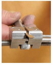
Narrower chisels cant slightly. Even in the jaws meant for chisels, narrower chisels would cock slightly out of square. As long as you're aware of it, however, this is easily compensated for because the guide's narrow wheel helps direct pressure.
