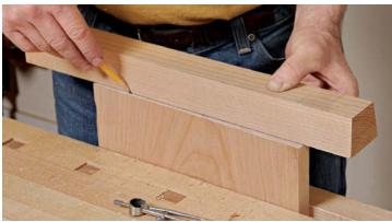
**Connect the dots.** To finish laying out the key's taper, use a straightedge and connect the divider marks.
