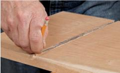
**Pencil lead reveals high spots during test fits.** When you're ready to fit the joint, pencil some lead onto the angled wall of the socket (left). When you push the joint together and it seizes (center), the lead will rub off on the high spots of the key (right). Plane these down.
