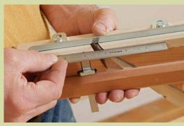
Hammer adjusts depth of cut. Tap the blade to advance the blade, and tap the body to retract it.
