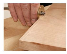
Scribe the key's baseline. Use the same marking gauge setting you used to mark the depth of the socket.
