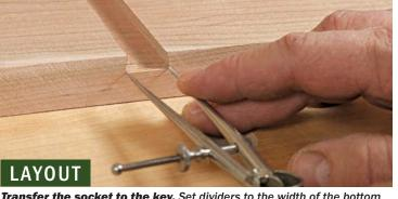
**Transfer the socket to the key.** Set dividers to the width of the bottom of the socket at the front and back edges of the shelf (above). Make prick marks to transfer these dimensions to the ends of the shelf (right).
