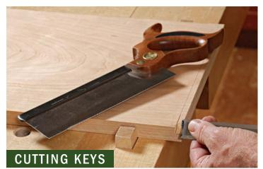
**Relieve the front corner.** Because he must plane across the grain to create the key, Gochnour cuts and chisels off the front edge to prevent blowout (which could be caused even by the plane's scoring cutter).
