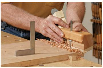
**Plane close to the pencil line.** Because the key tapers, you'll take more passes at one end than the other, using the layout line as a depth guide. Keep a square handy to make sure the plane isn't tilting.
