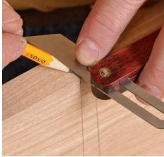
Bottom is angled. Grab a bevel gauge, set to the angle of your dovetail plane, when wrapping the bottom line onto the edges of the workpiece.
