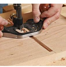
**Start sawing.** Just as it did for the through version, the batten serves as a guide while you saw the walls of the stopped dovetail. After chiseling out most of the waste, bring the socket to final depth with a router plane.
