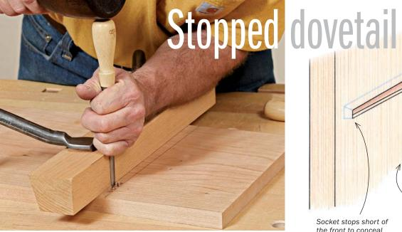
**Stopped socket starts with mortise.** A mortise at the front of the socket provides a place for the saw's toe when sawing the socket walls.
