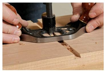
**Router plane finishes the socket.** While a chisel can level the joint, a router plane is more efficient and reliable.
