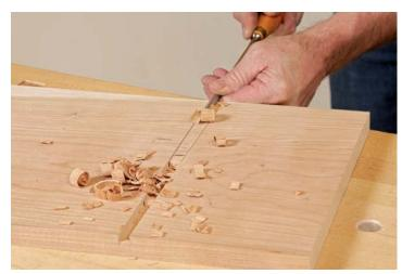
Pare most of the waste. Work in from both edges to prevent blowout.
