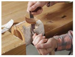
Debark. As you work to the exterior lines, start with a small drawknife before moving to a spokeshave or block plane for finer cuts. But don't go all the way to the line yet. Leave material for finishing cuts after the blank has dried.
