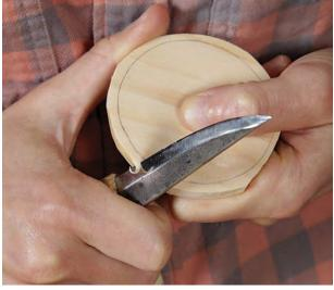
As it dries, the circumference of the pot will shrink to create a tight fit between the walls and the bottom.
