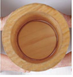
**See the light.** The bottom should audibly pop into place, but you still want a gappy fit. This allows the pot to shrink around and capture the bottom without splitting.
