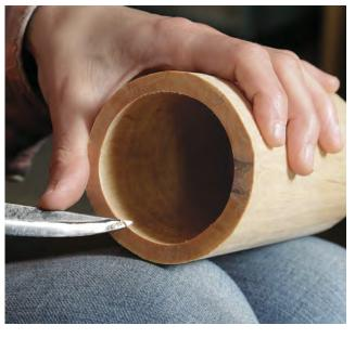
Chamfer the inside of the top. Byrd uses her sloyd knife to break the sharp edge within the shrink pot, pressing the blade with her thumb for a fine, controlled cut.
