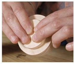
Checking the fit of the lower lid is a slow process, so take your time. If it's done well, you can achieve a twist-lock fit, where the lid locks when turned. After the lower lid fits, you can glue it to the upper lid. While the glue is still wet, though, carefully put the lid onto the pot and gently shift the upper lid to line up with the outer walls of the pot.
