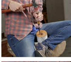
Chisel away the remaining bulk. If your bit's too small to drill out all the waste, use a mallet and a stout gouge with a deep sweep to approach the lines. Byrd sits to clamp the pot with her leg, allowing her to reposition the vessel quickly and easily.
