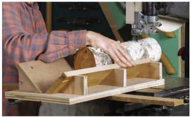
**Cut the blank and mark the diameter.** Byrd uses a V-sled at the bandsaw to cut the wet rounds to length. Then she scribes the inner and outer diameters using a compass. Aim for the shrink pot's walls to be an even %-in. thickness. Uniformly thick walls allow the pot to release moisture evenly as it dries, reducing the chances of cracking.
