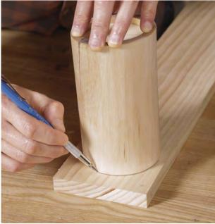
Glue and center the lid. After fitting the lower lid, apply glue, align the marriage marks, and hold the parts together until they stay adhered but can still move. Lower the lid onto the pot with the marks aligned and then gently slide the upper lid flush with the pot's walls. Remove the lid and clamp its two parts together with a weight.
