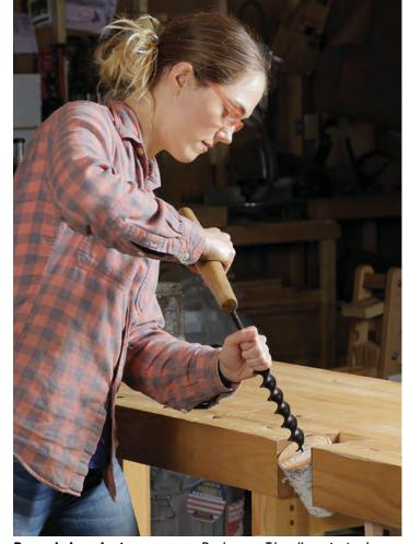
**Bore a hole as large as you can.** Byrd uses a T-handle auger to clear as much waste as possible. She sights straight down the bit to make sure she's parallel to the blank. If there's a kink in the round, she bores from both ends.
