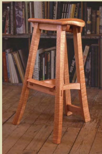
Multiplication is no problem. On one job for a home in southern Florida, Gilpin built 14 of his signature bar stools in 13 different woods, most native to the region. For the cutlist, one quick drawing and a short list of parts did the trick for all of them. He simply added a vertical column to the right of the grid for each additional species, enabling him to check off and keep track of the scores of parts.
