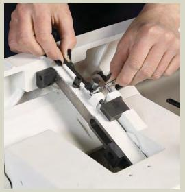
**Fence should be simple to set and lock tight.** A jointer's fence needs to be easy to square (left) and should stay there when locked. While every jointer had a 90° stop for the fence (right), not all were reliable, and would lose their setting.
