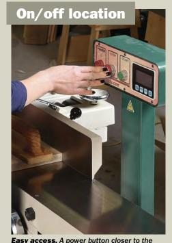
**Easy access.** A power button closer to the cutter means it's easier to turn off a machine midcut if something goes wrong.
