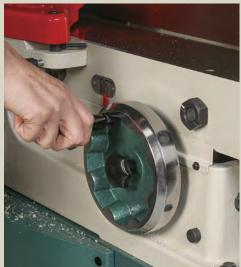
Wheels over levers. Some jointers rely on a wheel to adjust the height of the infeed table: others use a lever. Kaspern prefers the wheel because it lets you make finer adjustments with more precision.
