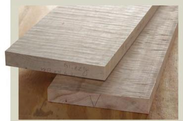
Smooth results. Spiral cutterheads leave smoother surfaces than straight knives, even on curly maple. In our tests, when there was tearout, it was minimal and localized.
