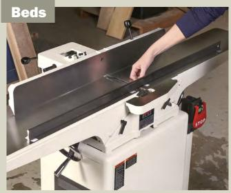
Beds must be flat. When setting up each jointer, Kaspern used a long straightedge and paper shims to ensure the infeed and outfeed tables were coplanar.
