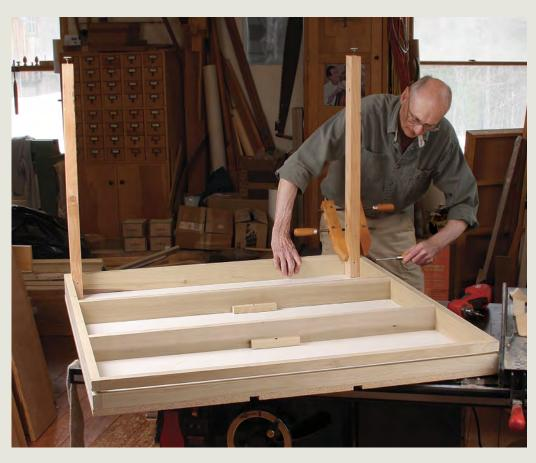
joint at the intersection for stability, and screw the cross-braces between the legs.
