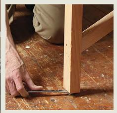
**Sight and set.** Use a long straightedge to sight along the length of the tablesaw top and the outfeed tabletop. The front edge of the outfeed table should sit just below the tablesaw top. Set the levelers accordingly. The levelers have a square or hex head just above the pad. Use a crescent wrench to adjust them up or down as needed.
