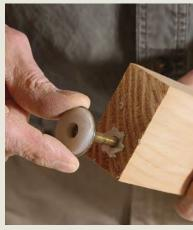
Make legs and add cross-braces. Before you screw the leg in place, drill and tap in a T-nut and add a leveler to the bottom of each leg. These will help you level the outfeed table to the saw table. Mark the first cross-brace in place (bottom right), cut it to length, and screw it to the legs.
