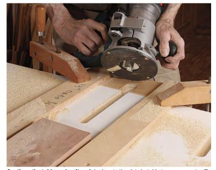
**Continue the tablesaw's miter slots.** Locate the slots by taking measurements off the tablesaw and drawing them on the outfeed table. Using a 1-in. router bit builds in some forgiveness when aligning to the saw's <sup>3</sup>/<sub>4</sub>-in. miter slots.
