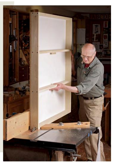
Measure from the edge of the tablesaw to locate the slots. Cutting the slots with a 1-in. router bit gives me a bit of leeway when aligning them to the tablesaw's 3/4-in. miter slots.
