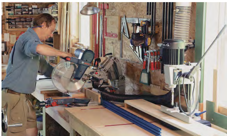
Miters and mortises. One run of counter accommodates Bauer's chopsaw and his hollow-chisel mortiser, which can be pulled forward for use.
