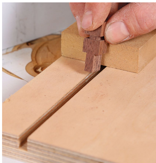
Simple fixture holds the post. Press the post blank into a grooved piece of plywood until it bottoms out. The stop stabilizes the blank.
