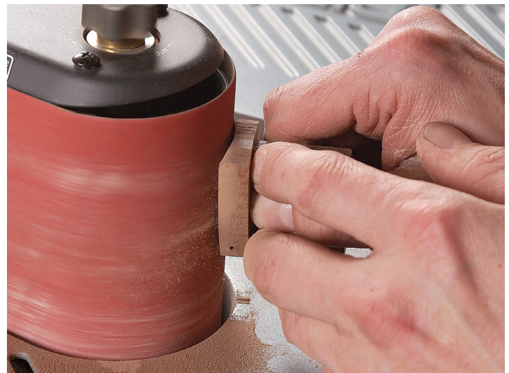
Hollow the back. Morley uses the large end of an edge sander to create a comfortable hollow.
