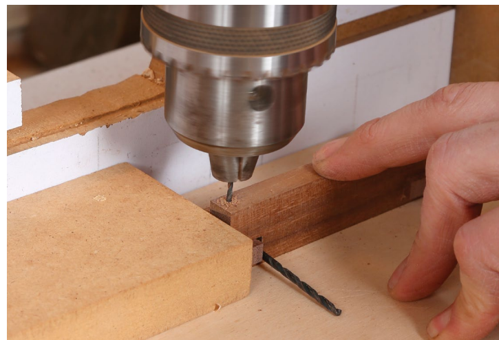
Drill for the pin. Fit the post and pendant blank together using a \frac{1}{16} -in.-dia. drill bit as a spacer. Push the pendant blank into the groove and against the stop (left). Then drill a \frac{1}{16} -in. hole through the pendant and post (above).
