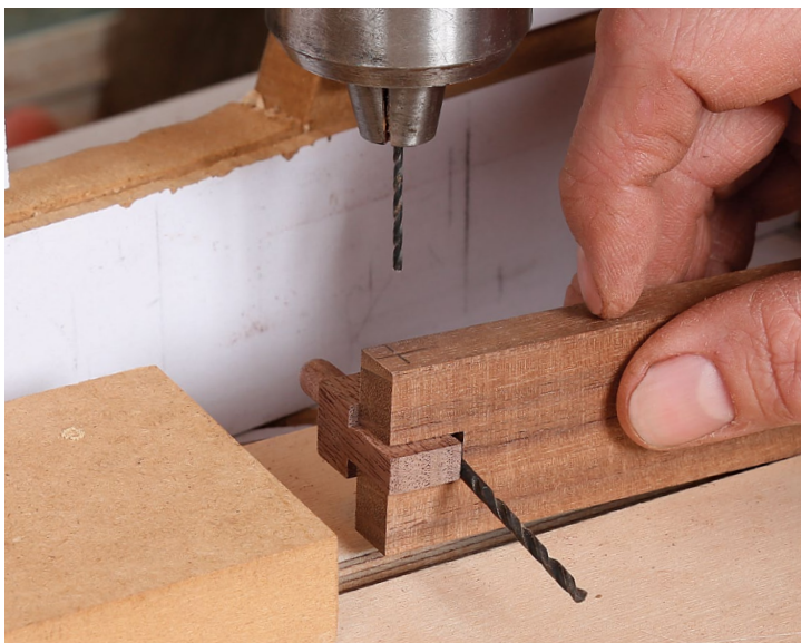
Simple fixture holds the post. Press the post blank into a grooved piece of plywood until it bottoms out. The stop stabilizes the blank.
