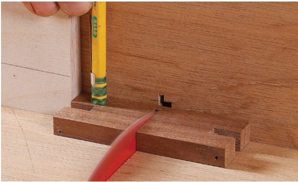
Cut the pendant blank in two. A stop ensures that all of the individual pendant blanks are the same length.
