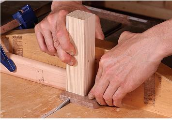
**Dado for the bottom.** Once cut to length, the staves each get dadoed to receive the bottom.
