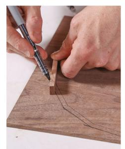
**The cut line gets enlarged.** Make a spacer whose thickness is somewhat less than the depth of the dado for the bottom.
