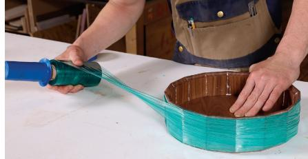
clamping. Blue tape provides the initial hinging and clamping action, but then Lutz circles the tray many times with stretch wrap, which exerts excellent clamping pressure.
