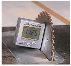
Digital assistant. With so many staves in a vessel, dialing in the bevel angle is critical. Lutz uses a digital angle gauge at the tablesaw and the jointer. For safer machining, he does the beveling with the staves still in long blanks. Each long blank yields three staves.
