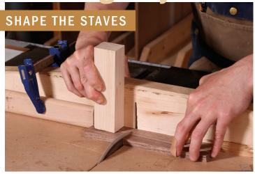
**From triple to single.** With the bevels perfected, crosscut the staves to final length, three per blank.
