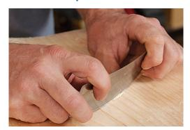
**Stand up straight.** Galbert finds the optimal scraping angle by starting at 90° to the work and gradually tilting the scraper into the direction of cut until he gets a shaving. It should still be nearly vertical when you are cutting.
