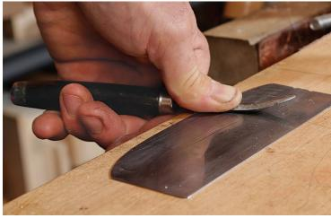
**Turn a burr with a burnisher.** Using firm pressure and a few drops of oil, press a burnisher across the face of the scraper (above). Then hold the scraper upright and, using moderate pressure, draw the burnisher along the edge to create a burr (right). The burnisher should be tilted just slightly downward toward the side that is getting the burr.
