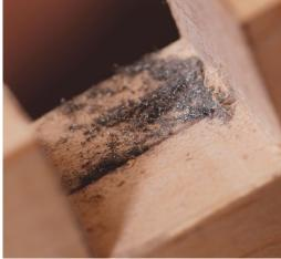
File comes first. With a fine file held flat to the bottom of the notch and at a skewed angle, cut by drawing the jig and file toward you (left). Use a light touch. When you've filed into fresh metal you should be creating curly strands of steel (above).
