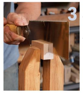
One slice for the scraper. Flip the jig upside down and cut a kerf to fit the scraper. The fit should be snug but still allow the jig to slide freely on the scraper.
