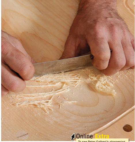
**Skewed logic.** Like other hand tools, the scraper cuts cleanly when the strokes are diagonal to the grain.
