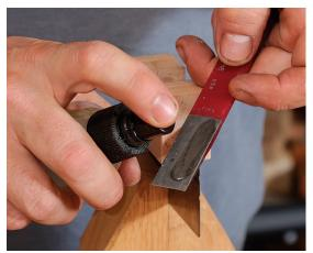
**Oil and diamonds.** After filing the edge square, Galbert uses a fine diamond hone lubricated with camellia oil to create a super-smooth surface.
