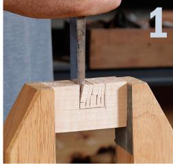
Rough out the notch. To create the jig's notch, start by cutting a handful of kerfs, then chisel out the waste.
