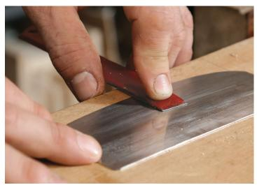
**Final flattening.** Use the fine diamond hone to flatten the face of the scraper, being careful never to tilt the hone. Then hone the edge again.
