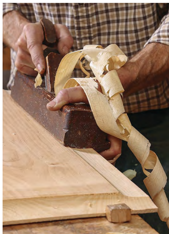
Plow around the field. Breed's plane cuts a slightly concave border to create a handsome fielded panel.
