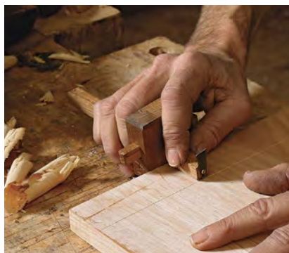
Preparing for the panel. The fence on Breed's antique panel-raising plane, set with two screws, controls the width of the border the plane cuts around a panel. Before cutting cross-grain, Breed scribes the edge of the border with a cutting gauge.
