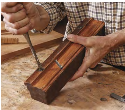
Preparing for the panel. The fence on Breed's antique panel-raising plane, set with two screws, controls the width of the border the plane cuts around a panel. Before cutting cross-grain, Breed scribes the edge of the border with a cutting gauge.
