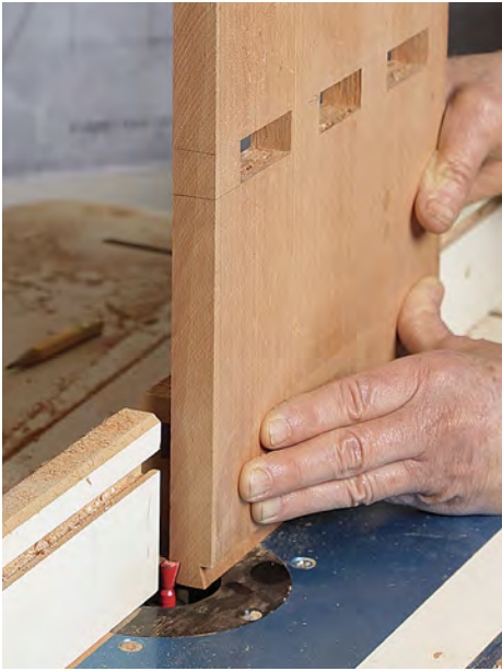
Sliding dovetail joins cornice to case. Before gluing the case together, cut the dovetail on the top of the sides. Each cornice will get a mating slot.
