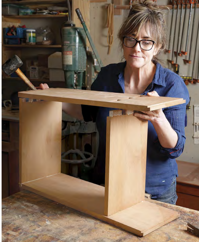
Glue the case. The bottom corners are dovetailed, and the shelf has through-tenons. It's not typical case construction, but it's quite strong and not difficult to manage.
