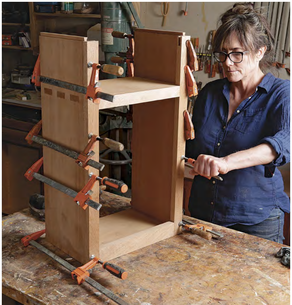
Add the face frame. Hiller first glues up the face frame, then glues and clamps the face frame to the case. The face frame is joined with mortise-and-tenon joints and slotted for splines that will link the fascia to it.
