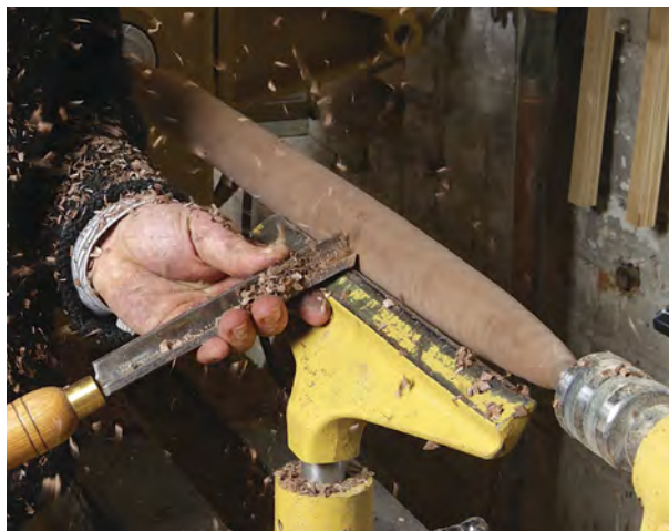
Turn and kerf. After turning the legs and stretchers, prepare the leg tenons for wedging by kerfing them on the bandsaw.
