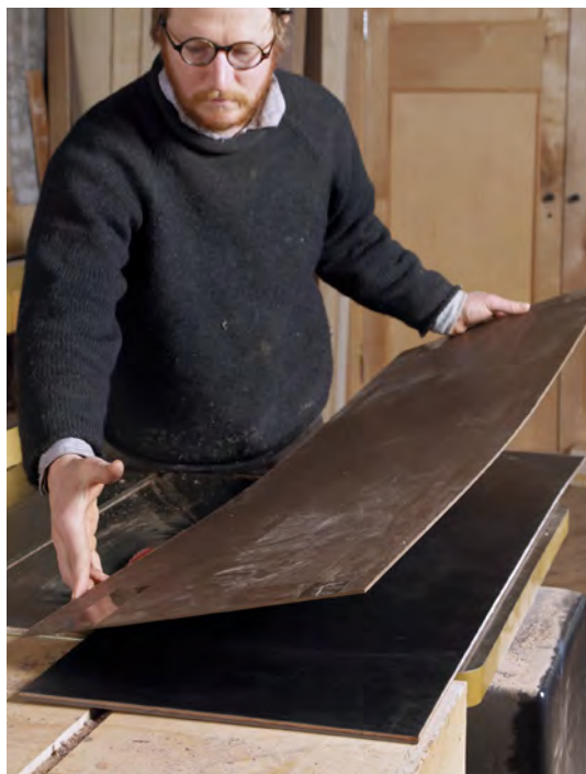
Cut the blotter to depth. With the leather glued to the Masonite backer, sandwich the leather with another piece of loose Masonite, and rip to final width.
