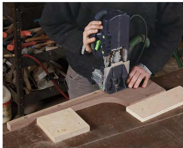
Mark and cut Domino mortises. Dry-fit and clamp the case parts, and mark the mortise locations. Then cut the mortises.
