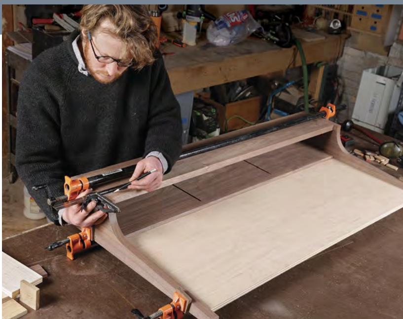
Mark and cut Domino mortises. Dry-fit and clamp the case parts, and mark the mortise locations. Then cut the mortises.
