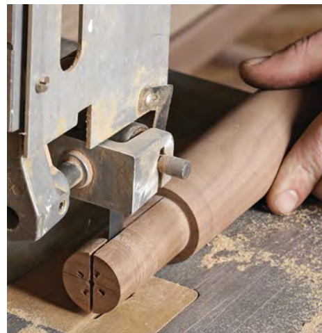
Turn and kerf. After turning the legs and stretchers, prepare the leg tenons for wedging by kerfing them on the bandsaw.
