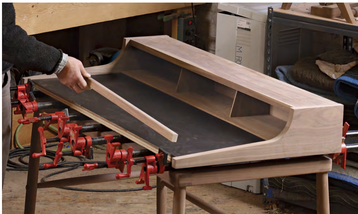
Add a lip. Cut a solid-wood lip for the front of the desk. It will obscure the edges of the plywood and the blotter. Remove the blotter to glue on the lip, then reinstall the blotter.
