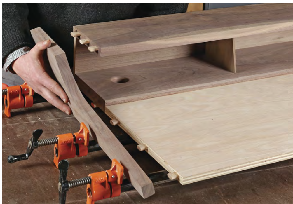
Final assembly. After setting the gallery back and drawer dividers in place, fit the gallery top (left). Then add the end caps (below).
