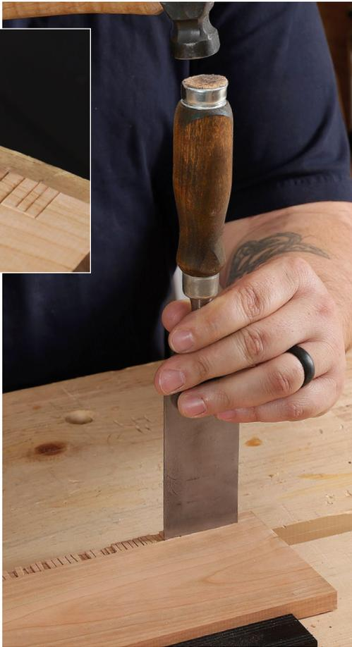
**Sever fibers at the back.** Place a wide chisel (1 in. or wider) in the line cut by the marking gauge and give it a good whack.
