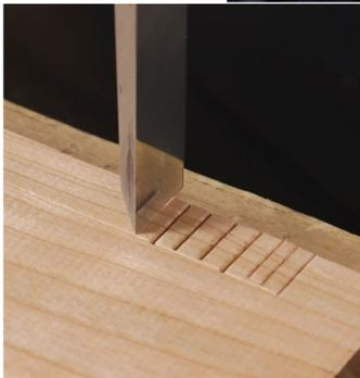
**Break up the waste.** After laying out the rabbet with a marking gauge, work your way along its length with a chisel, cutting across the grain.
