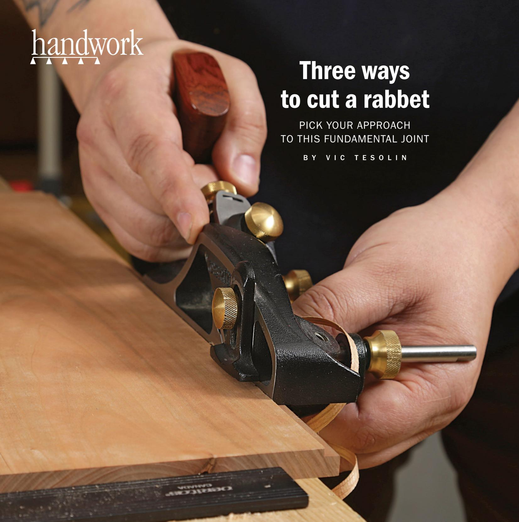
**A**lthough not as glamorous as the dovetail nor as robust as the mortise-and-tenon, the rabbet joint is just as useful. It shows up in casework as a place to put a frame-and-panel back, and is a popular way to fit a drawer bottom into its grooves. So it's a good joint to learn. In my shop, where I depend on hand tools to cut all joinery, I've employed three approaches to cut rabbets. For through-
