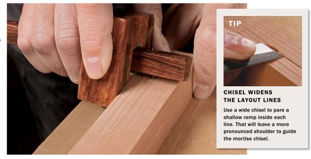
Mark the tenon shoulders and cheeks. The pin-style gauge works well to mark the tenon cheeks (right) in end grain. But Miller marks the shoulders with a disk- or knifetype marking gauge, which works better cutting across the grain. The tiny bevel faces the waste wood, leaving a square cut at the shoulder.
