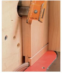
Fine-tune the machine setup. At the tablesaw use the pencil lines as a guide (left), but dial in the fit by testing the tenon in the mortise (below). Now you can cut other tenons with the same settings.
