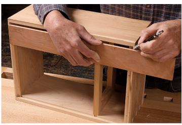
**Mark in place.** Miller fits one end of a backboard into its rabbet and uses the opposite rabbet to mark the far end of the board.
