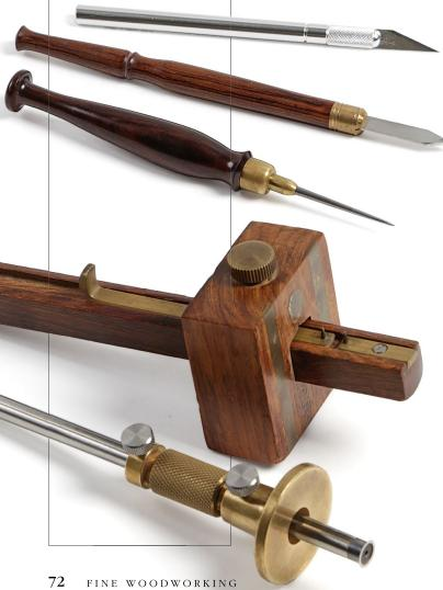
The other useful pointscribing tool is a scratch awl. I use mine to transfer a dovetail layout from one part to another. I find this task easier with an awl than a knife, since there is no tendency to cut into the part you're marking from. To transfer dovetail marks around the workpiece, however, I use a flat-sided marking knife.
