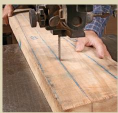
**Cutting it close enough.** Follow the rough lines on the bandsaw. These cuts don't have to be perfect. Make crosscuts with a miter saw or circular saw.
