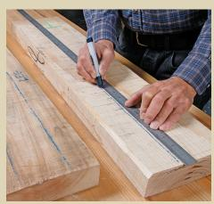
**Bold lines of attack.** Mark out parts on the rough boards with a lumber crayon or fat pencil, factoring in extra length and width. Use a long ruler to align parts with the grain.
