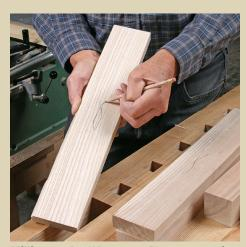
**Milling marks.** When you mill parts, use a fat pencil or a crayon to mark reference faces.
