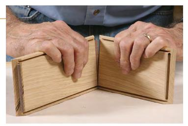
**Dry run.** Before glue-up, slip the splines into place and bring the corners together to check for gaps. Make sure the splines don't bottom out and prevent the miters from closing.
