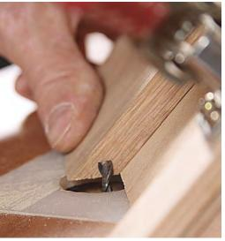
Where to rout. With the stock in the jig, Stowe eyeballs where to locate the fence. He aims for the bit to be roughly centered in the stock and always leaves at least ½ in. of clearance between the slot and the inside face of the workpiece.
