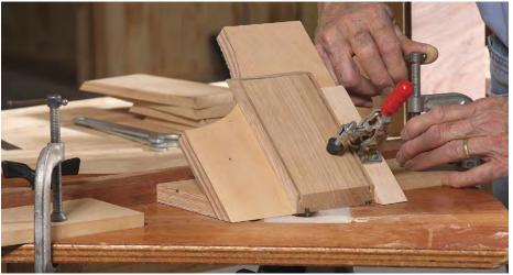
**Set the stops.** To accurately set the fence and the stops, temporarily mount the workpiece with the inside face out, so you can locate the stops referencing off the mitered face. If your box has grooves for the lid and bottom, locate the stops so you don't rout into them.
