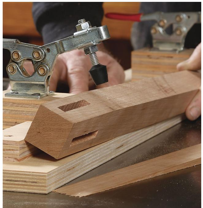
**Rotate clockwise.** This ensures you have square surfaces referencing on the jig's stops and platform for both taper cuts. Be sure to save the offcut for the second cut.
