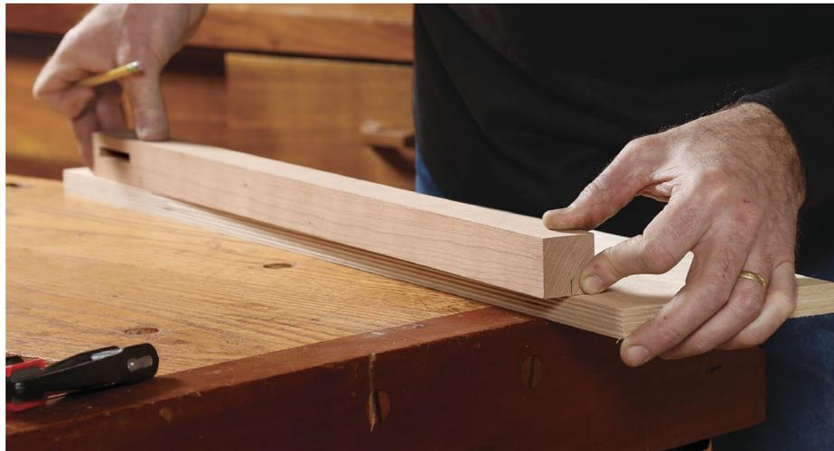
**Mark the taper.** On a square leg blank cut to length, mark the ends of the taper on a face and the bottom (top). Using the marks you just made, place the leg on the jig platform so the offcut overhangs the jig and the top of the leg is at the leading end (above). Then clamp the leg in position.
