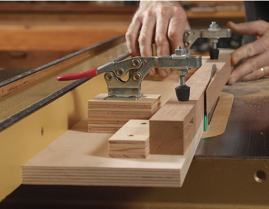
**Time to taper.** As with any standard rip at the tablesaw, keep the sled tight to the fence. McLaughlin likes to use the nearer clamp as a handle for good control.
