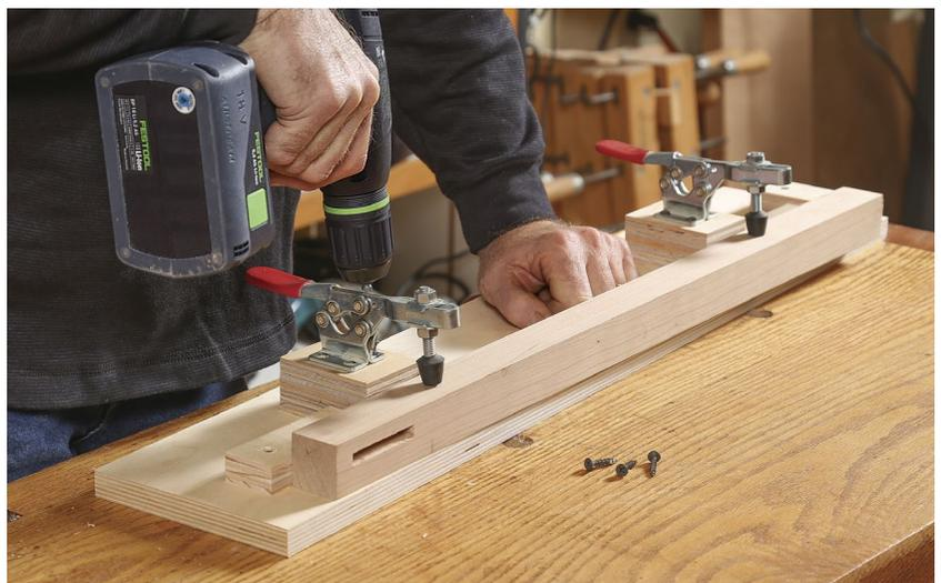
**Add stop blocks and hold-downs.** Three stops—one at the leg's foot and two flush with its side—are all you need for repeatable cuts. Toggle clamps screwed to riser blocks keep the leg secure as you feed it through the cut. Just make sure to get the right amount of clamping pressure. Too little, and the leg may slip during the cut, but too much may force the leg out of square.
