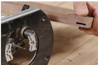
Set the stops. Morgan's jig allows him to limit front-to-back and side-to-side travel, keeping his router on track. Because his magnets are 1/8 in. thick, Morgan uses a 1/8-in. solid carbide spiral bit. The magnets are 3/4 in. dia. and he cuts the mortise 7/8 in. deep to leave a little room for a plug.
