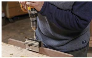
**Drill the rail.** Morgan relies on a doweling jig to help him drill square to the board. Tape on the bit acts as a depth gauge. You want the top magnet to sit flush with the surface.
