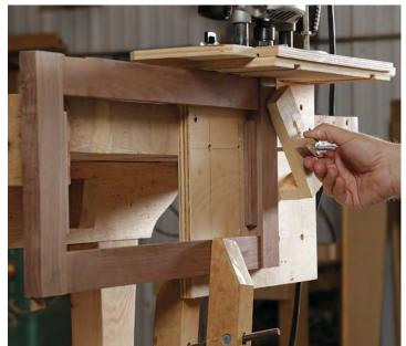
Clamp the door in place. Morgan first clamps the door tight to the bottom of his jig's platform with a wooden hand screw, then tightens the main clamp.
