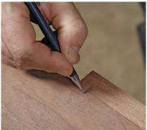
**Determine where to install the magnets.** Sticking the smaller magnets to the one in the door lets you easily mark their centerline on the top of the door. All you have to do after that is line up the door with its final position on the case rail and transfer the mark across. Measuring works, too.
