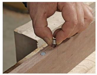
**Drop and cover.** After placing the magnets inside, glue on the shopsawn veneer strip. Morgan uses a clamping caul with clear packing tape on one edge.
