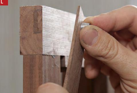
**Magnet test.** To determine the number of magnets you'll need in the carcase, hang the door, hold a stack of magnets behind a veneer strip, and approach the magnet hidden in the door. You want their attraction to engage when they're about  $^{3}/_{4}$  in. to 1 in. apart.
