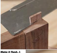
fine-tooth pull saw and slicing cuts with a sharp chisel make quick work of the extra length, leaving you with a clean, flush surface on the frame.
