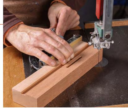
**Miter the back corner.** After cutting a slot for the bolt, clip the back corner of the fence at 45°.
