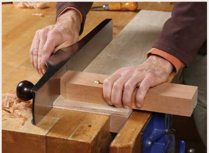
locked in place with the bolt. I always set the fence so that it overhangs the edge of the base just a fuzz. I then use my plane to shoot it flush to the edge of the base, creating a zero-clearance fence that prevents tearout when you trim end grain.
