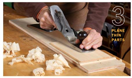
After removing the fence, you can use the low stop for planing boards as thin as <sup>3</sup>/<sub>16</sub> in. thick. The base provides a stable, flat planing platform.
