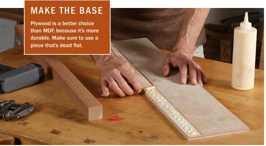
**Glue for the rabbet.** The rabbet's short shoulder is tall enough to register the cleat parallel to the edge of the base, while the glue creates a strong bond that prevents the cleat from shifting in use.
