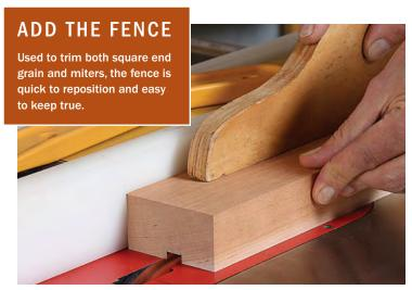
**Groove the fence to fit the stop.** Set the rip fence to cut a groove down the middle of the fence. The blade's height should be the same as it was for the dado in the base.
