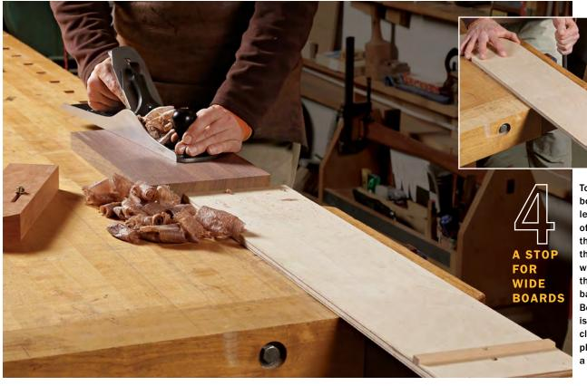
To face-plane wide boards, slide at least half the base off the bench and then clamp it in the vise. Set the workpiece against the end of the base and plane. Because the base is low, you won't clip it with the plane at the end of a stroke.
