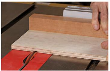
**Cut a dado for the stop.** It's doesn't need to be deep— $\frac{3}{16}$  in. works great. Locate it 2 in. or so from the end.
