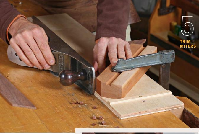
When shooting miters, there's always a danger that the plane will pull the workpiece forward as it cuts. The solution is to take smooth, easy passes. Thin shavings are better than heavy ones, too, because it takes less force to make them.
