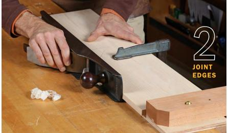
With the end grain against the fence, you can also shoot long grain. Rousseau clamps the workpiece to the base to help stabilize it. Because breakout isn't a concern, the part can overhang the edge and fence.
