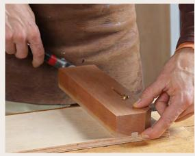
Zero-clearance fence. Set the fence just a hair over the base's edge. Rousseau does this with the bolt snug, tapping the fence's other end with a mallet (above). Then plane the fence flush to the base's edge (right). This prevents tearout on the back edge of the workpiece.
