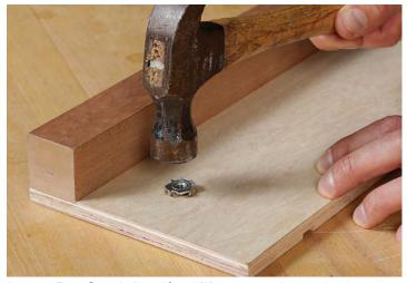
**Insert a T-nut from below.** After drilling a counterbore and a throughhole, hammer in the nut from the bottom.
