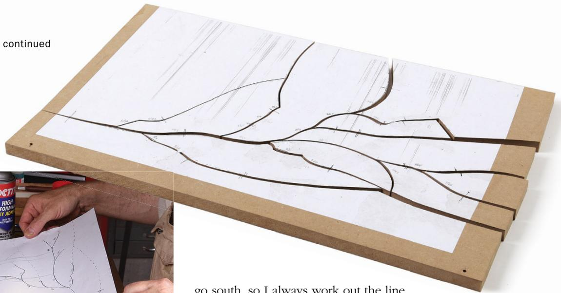
go south, so I always work out the line thicknesses, intersections, and cut sequences on a test piece of ½-in. MDF. If that goes well, I repeat the process on a slab of hardwood, making any changes indicated by my first attempt. Once I feel comfortable, I do the actual piece. If I haven't had a successful attempt on a test piece, what insanity would make me believe it will magically come together on the real piece?
