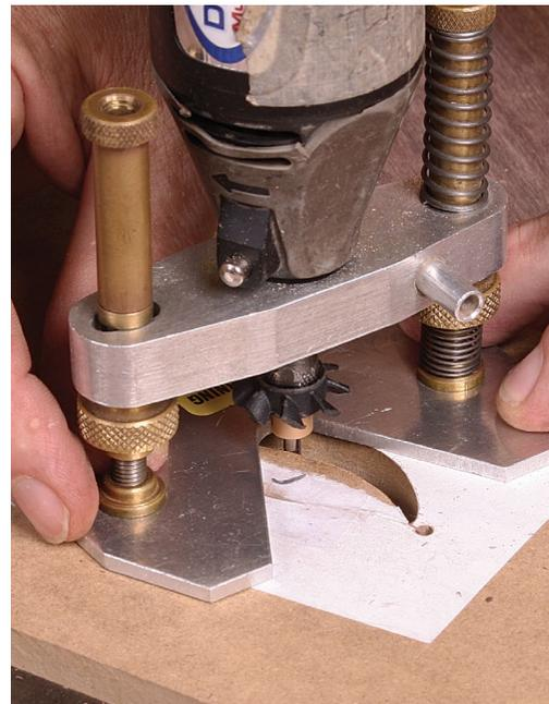
**Position the leaf.** Clamp the template on the workpiece where you want the leaf, put in the insert (above), and tape it in place. Then rout the center vein (left), inlay the stringing, and trim it flush. Repeat the sequence for each outside edge of the leaf (below).
