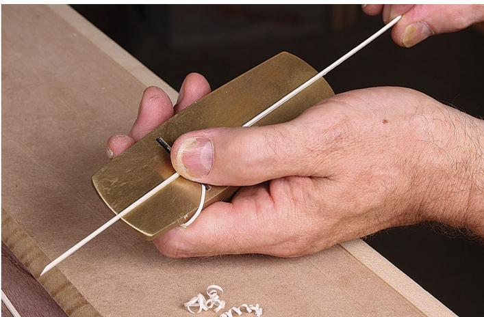
**Taper the strips.** The strips can be tapered with a small block plane. Pull the strip across the blade. There is a lot of fitting and trial-and-error here. Be prepared to break some strips and have to redo them.
