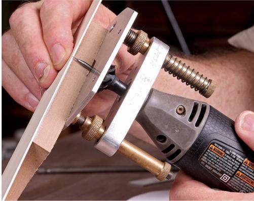
**Hands-free start and stop.** Latta uses a Dremel mounted in a Stewart-MacDonald router base and equipped with a foot switch for on and off (right). He starts by cutting the narrowest grooves (below).
