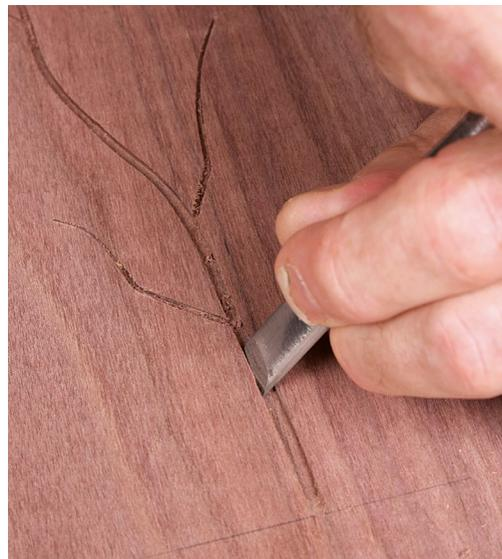
**Smooth the transition.** When moving from one width to the next, sand or chisel the edge of the groove to smooth the transition. Keep in mind that the shoulder between segments is only  $\frac{1}{32}$  in.
