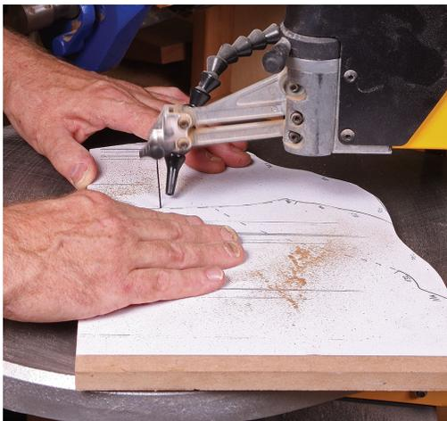
**Proper positioning.** The bottom piece of the pattern aligns the entire form. Latta installs a couple of registration pins along the bottom segment so that he can remove and remount it in the same place on the workpiece. On the blanket chest, these pins were positioned so the holes fell under its waist molding.
