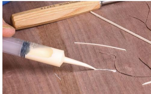
**Glue it in.** Once the stringing fits, glue it in using yellow glue. Latta uses a Monoject 412 syringe to put glue in the channel, and presses in the stringing with a metal ruler.
