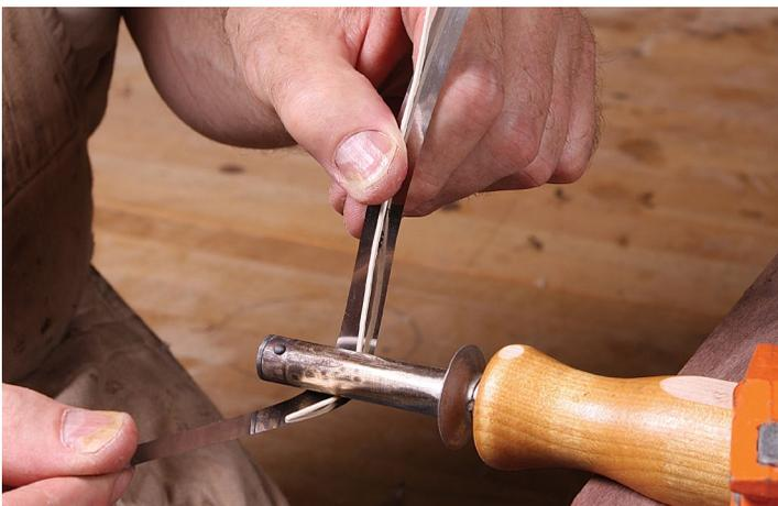
**Heat helps manage tight curves.** If there are any tight curves, bend the stringing on a hot pipe before you glue it in place.
