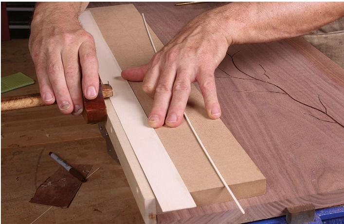
**Cut the stringing.** Using a slicing gauge with a shopmade fixture (MDF with a small lip attached), butt the stringing to the lip and start slicing at the bottom, working your way to the top. For a cleaner edge, cut halfway through and then flip the material and finish the cut from the other side.
