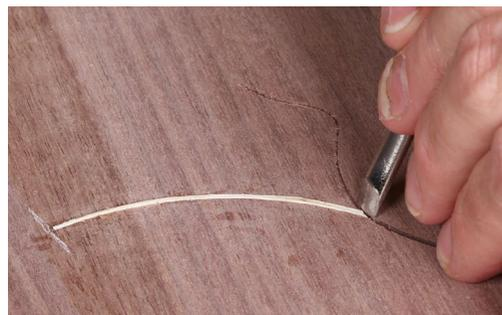
**Run through intersections.** Glue in the stringing so it lands beyond intersections, and then use a chisel or a gouge to cut it back to perfect length.
