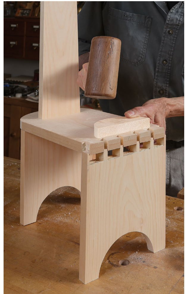
Mortise and dovetails first. Before applying glue, Becksvoort slides the back leg through the mortise in the step and just barely engages the dovetails at the front. He adds glue only to the dovetails and hammers them home.
