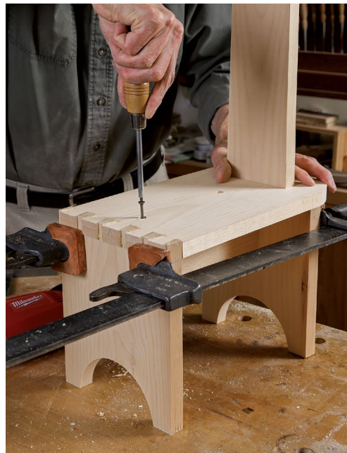
Add the arched brace. Clamp the brace in place, and then screw it in and plug the holes.
