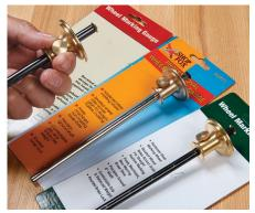
**Three of a kind.** Wheel gauges from Woodcraft, Rockler, and Shop Fox look similar to the IGaging gauge and have the same loose fit between fence and beam. But they lack an O-ring, making adjustments more difficult.
