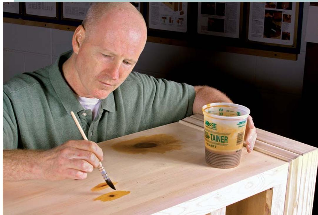
**Seal with shellac.** To prevent resin from staining the finish in the future, seal all knots and sap pockets in pine with dewaxed shellac.
