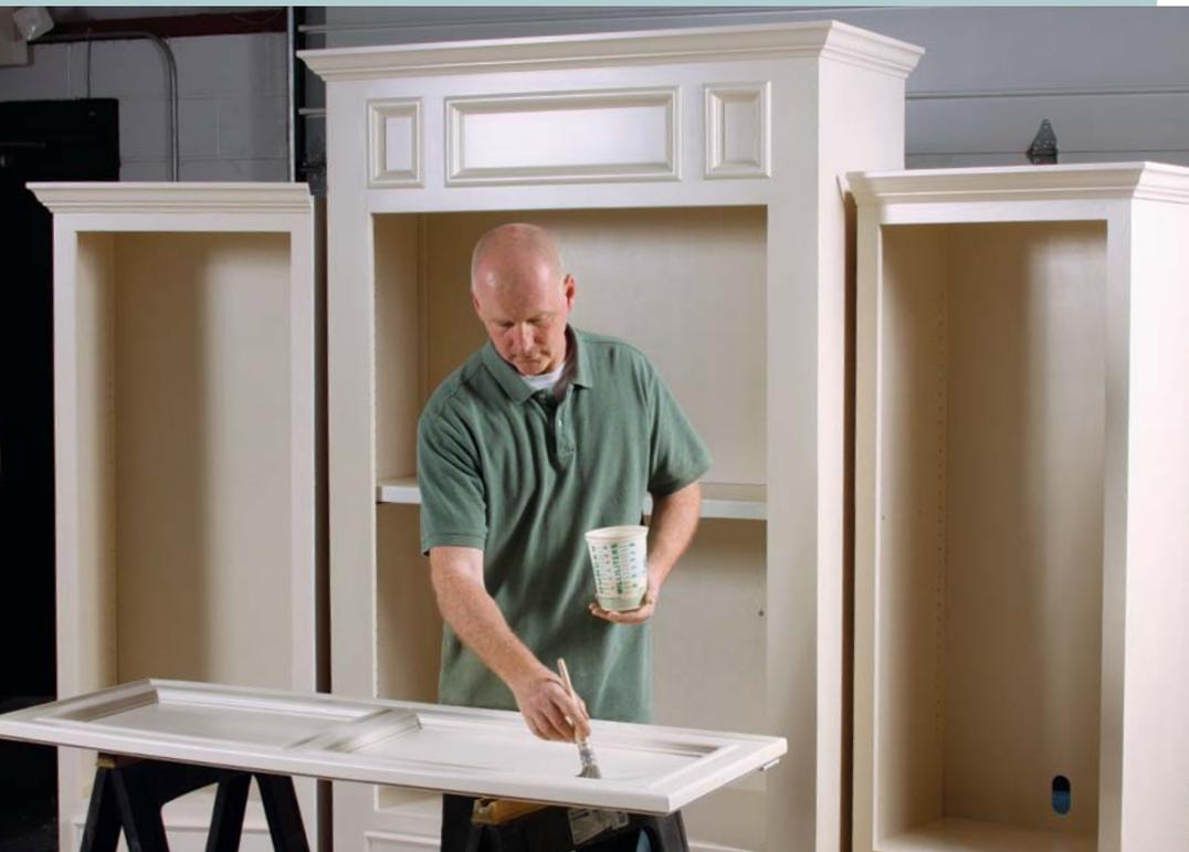
**Work horizontally.** On large and small pieces, when possible, work on a horizontal surface to reduce the risk of runs.
