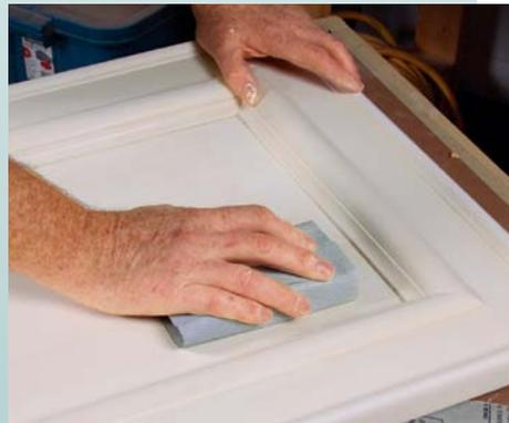
**Sand between coats.** Sanding not only removes dust nibs and brush marks, but it also creates a mechanical bond between layers of finish.
