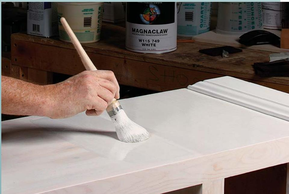
**Next coat.** After the first coat is dry, apply the second coat of primer with the same technique, but perpendicular to the first to reduce the buildup of brush marks.
