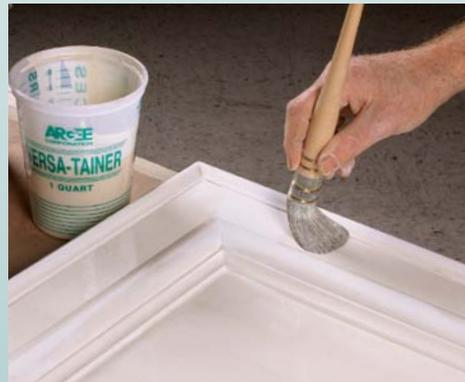
**Brush in sequence.** When finishing complicated surfaces, do the large surfaces first with a big brush, then cover molding and trim with a smaller one.
