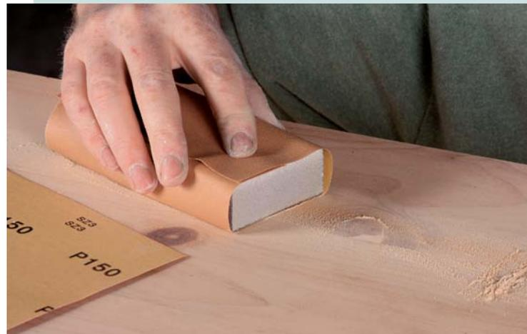
**Sand it flush.** Use P150-grit paper wrapped around a cork-faced block or a sanding sponge to level the filled area.
