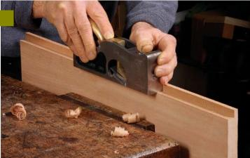
**Keep it upright.** For the wall parallel to the board's face (left), clamp the board between benchdogs and use your off hand to keep the plane tight against the rabbet's vertical wall. Use a vise for the other wall (above). With the board on edge, there's no need to lay the plane on its side.
