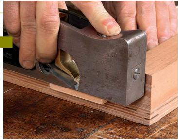
**Two steps for straight cheeks.** First, place the toe of the plane on the tenon and slide it forward until the blade just touches. Then take a shaving, keeping even pressure on the plane throughout the cut.
