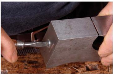
**Set the blade in the body.** Pinch the blade between your fingers to center it, and tighten the hold-down to keep it in place (left). Then adjust the mouth, if that's possible on your plane (above).
