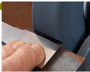
**Grind to the line.** Set the tool rest at 90° to the wheel. Grind away most of the excess, then smooth the rough edge on your sharpening stones.
