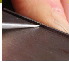
**Mark the sole's width.** Lowe uses the scribe from his combination square, holding its tip slightly above the plane body as a precaution against grinding the blade too narrow.
