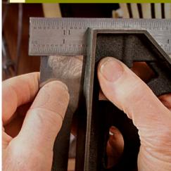
Look into the light. Register the square on the factory edge of the blade (the one you didn't grind). If the cutting edge is out of square, regrind it.
