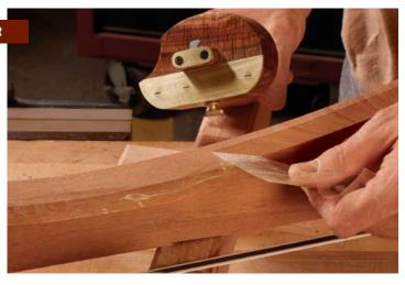
Apply the veneer. For both rails and dividers, use a cutoff as a caul, but add a piece of thin foam to even out the pressure between the curves. Cover the foam side facing the veneer in clear tape to prevent it from sticking to any squeeze-out.
