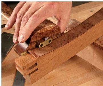
**Slice through the veneer.** After the glue has set on the lower rail, and with the gauge still set to the width of the banding, slice through the bottom part of the veneer.
