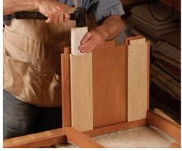
Let the sides move. The outer mahogany side is joined to the legs with elongated mortises to allow for movement. Use white glue, which also allows for movement. The internal poplar side rails are tenoned into the legs for added strength.
