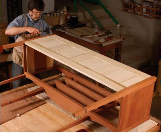
**Add the back.** Assemble the back separately by gluing the rear legs to tenons in the upper and lower rails and to the outer edge of the end stiles. Then glue the back assembly to the rest of the piece as shown, fitting it onto the outer and inner side tenons.
