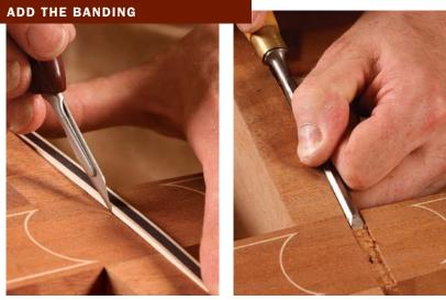
**Dry-fit the banding.** Place the banding in its groove and score the legs where it crosses them (above left). Make several cuts across the legs with a sharp knife and then remove the waste with a chisel (above right) or a router plane.
