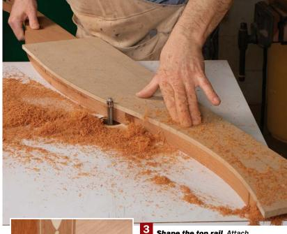
Shape the top rail. Attach the template to the bandsawn top rail and trim it flush (above), stopping just over halfway to flip the workpiece and reattach the template to rout the rest of the profile. Then dry-fit the legs and check that the upper rail is set back just enough to leave the veneer slightly proud of the leg (left).
