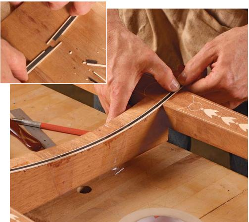
**How to splice it.** There is no natural place along the front to hide a joint in the banding, so create a staggered splice (inset). Clear tape is sufficient to hold the banding in place until the hide glue dries.
