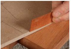
Make room for veneer. Make a half-template from the centerline over, and use it to extend the lines you just drew. Then pull back the template just enough to allow for the vertical-grain veneer that you'll apply.
