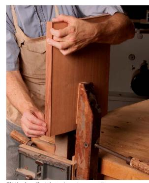
Fit the beading. A good way to secure the curved door without damaging it while you fit and then glue in the beading is to use a hand screw with cork-faced pads.
