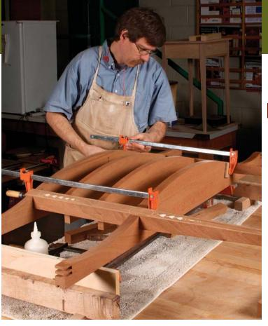
**Glue up the front.** It's finally ready. Glue together the front of the sideboard and add the extra pieces of vertical-grain veneer where the rails and dividers meet the legs.
