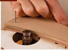
**Shape the cock beading.** A template curved on one side and straight on the other profiles the beading for the doors' top and sides.
