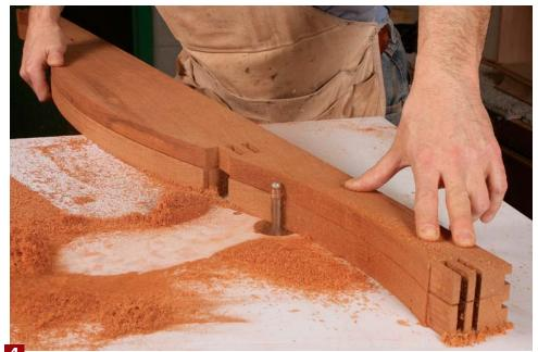
The rail becomes the template. Use the top rail to shape the lower rail and then the two drawer dividers to give all four pieces the same profile.
