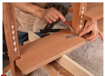
Where leg meets curve. With the front of the sideboard dry-fit, lay a straightedge across the front of each leg and mark where it meets the rails and the dividers.
