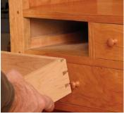
**They guide the drawers.** Tapering the runners has the same effect as tapering the case.
