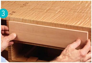
Now fit for length. Trim the right end just like the left, parallel to the opening. At this point, the fit should be tight.
