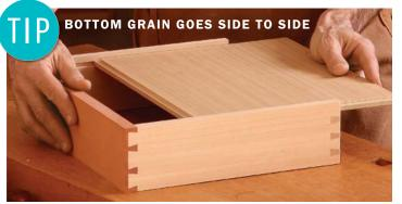
This is a must on a solid-wood drawer bottom, so when it expands, it doesn't push out the sides, locking the drawer into the pocket or worse, breaking the joints.
