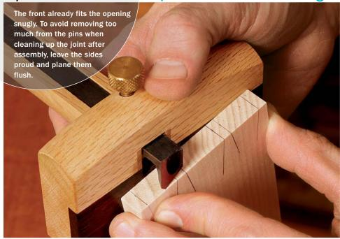
**Leave the pins a little short.** Set your gauge about ½4 in. shy of the side's thickness, and use it to mark the tails' depth on the drawer front.
