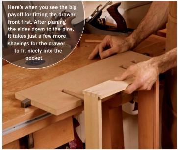
**Do the sides first.** This simple jig holds the drawer box much better than a vise can for this job. It's a piece of ¾-in.-thick MDF clamped between the benchdogs. The slots are spaced so the sides and the front and back can be planed. And you don't need to clamp the drawer in place.
