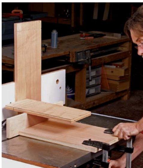
Watch the length. Make the base long enough to be clamped to the tablesaw's edge.
