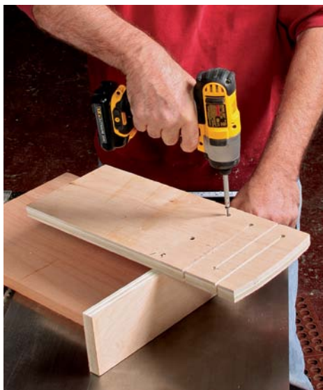
Start with a base. Two pieces of plywood make a solid foundation for a featherboard.
