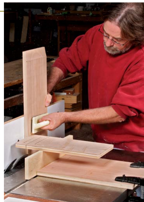
Keep it vertical. The featherboard keeps the panel pressed snugly against the fence.
