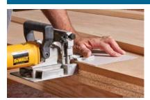
Biscuits align it. Van Dyke uses a shim to offset the biscuit joiner when cutting the slots in the top's edge. This ensures the edging will stand proud of the top for trimming flush.
