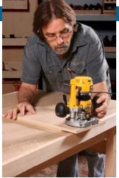
Trim the edging with a router. This simple base allows a straight cutting bit to trim the edging flush with the surface of the top.
