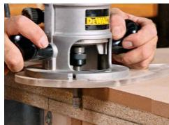
Assemble the top. Start with one layer cut to exact size, then use a router and flush-trimming bit to trim the adjacent layers.
