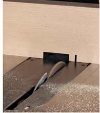
**Then the fence stays put.** Use a spacer block (left) to reposition the leg for cutting the dado's opposite end. Cut each wall cleanly, supporting the leg with the miter gauge, and then make passes to remove the material between them (right).
