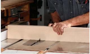
**First the fence gets set.** The rip fence will be your stop. Lay out one of the legs and set the fence so the blade lines up with one end of the dado.
