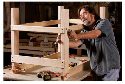
width and in exactly the same place on each leg. If you leave the crosspieces and stretchers a bit wide, you can edgeplane them in the thickness planer for a precise fit in the dadoes and rabbets.
