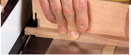
Tenon and slot the posts. You can form the tenons with a standard tablesaw blade. Use a miter gauge, with the rip fence as a stop. Work your way around the stock, making multiple cuts (above). Create the slot on the top of the posts with a tenoning jig (right).
