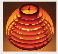
four curved, notched plywood frames get screwed to a top and bottom ring turned from a bricklaid block of cherry. When the rings are attached, they follow the stepped shape of the frames. The brass hanger is from Lampshop.com, with its ring snipped off and its arms inserted into the cherry ring. -C.B.
