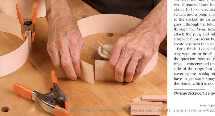
I glued into the rings (see photo, left). You might be tempted to just test-fit one ring for the outside and one for the inside and make the rest to match. I am leery of this method for two reasons. Test-fitting a circle on the inside is more difficult than the outside. If you don't get it right, you could mess up all the interior rings. Also, you could end up with squarish circles instead of the consistency you get with minor calculating.
