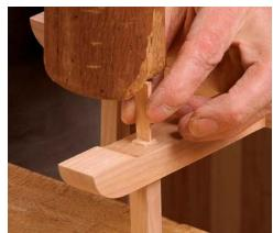
Glue the posts into the base. For added strength, Becksvoort hand-saws a kerf in the tenons and wedges them during the glue-up (above). So the top doesn't get in the way while gluing in the rings, he only dry-fits it at this point, holding it place with rubber bands (right).
