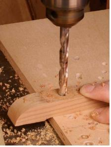
**Start on the drill press and finish up by hand.** While the base pieces are together, drill for the center hole that will hold the brass post (left). Then take apart the base and drill the four holes that will be the through-mortises (center). Use a chisel to turn the drill-press holes into square mortises (right).
