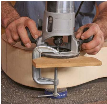
**The tools are familiar.** After using a router to trim the top flush with the sides, clamp on a shopmade fence (above) and use a straight bit to cut a very shallow rabbet in the guitar's side. Next, use multipurpose household glue (Duco cement by Devcon; \$5) to attach the plastic binding that protects and hides the joinery. Blue painter's tape clamps the binding into the rabbet (below). When the glue dries, trim the binding flush with a card scraper (right).
