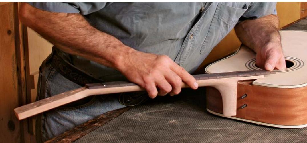
**A crucial joint simplified, but only a little.** In many kits, the neck attaches to the body with a couple of bolts instead of a dovetailed key. The dovetailed key is more traditional, but many makers use a bolt-on neck for ease of construction and repair. You may need to carefully sand the neck's heel to adjust the fit and ensure that the neck meets the body at the correct angle.
