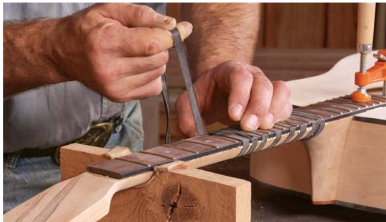
**Tip for attaching the fretboard.** With the neck temporarily attached, Vondriska uses a length of elastic from an old inner tube as a clamp when gluing the fingerboard in place.
