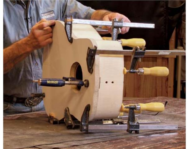
**How to avoid specialty clamps.** Gluing up the sound box typically requires 25 to 30 luthier's spool clamps for even pressure around the top. Vondriska uses a few ordinary bar clamps and a guitar-shaped caul to distribute pressure.
