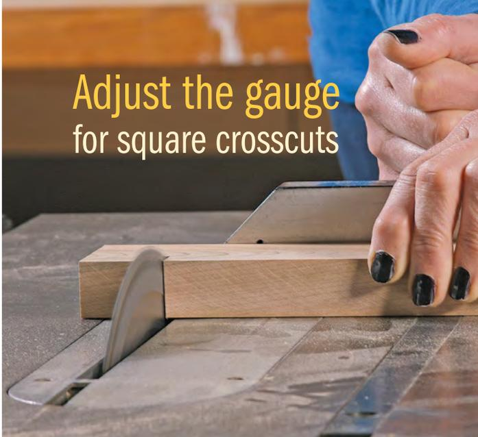
**Square the miter gauge.** No light should appear between the ruler's edge and the miter gauge's bar while the head of the square is tight to the fence. If it does, loosen the handle and fine-tune the setting.
