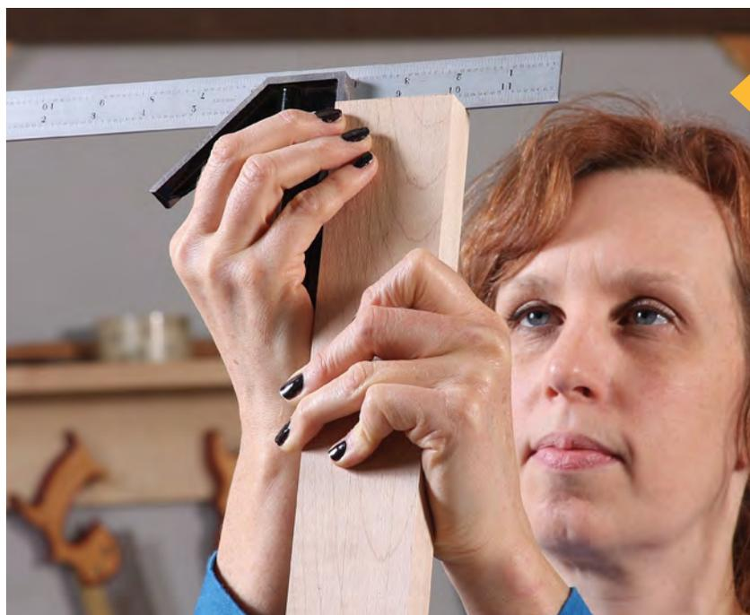
**Test cut confirms your setting.** Crosscut a piece of wood with two flat, parallel faces and one jointed edge. With the jointed reference edge against the miter gauge, run the wood through the saw and check the cut with a reliable square.
