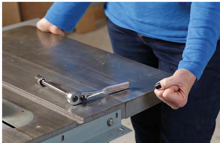
**Tap it home.** After loosening three of the bolts that attach the top to the cabinet, use the tight bolt as a pivot point to bring the miter slot into parallel with the blade.
