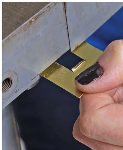
**Shim with brass to align the top.** To adjust the top, place one or more notched brass shims around the bolts that secure the tabletop to the base. Remember to retighten the bolts afterward.
