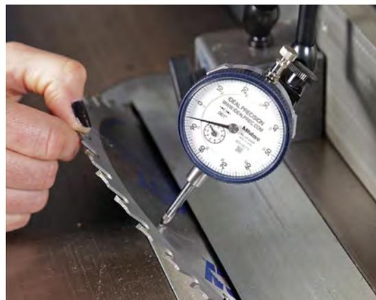
**Measure at the front and back.** Move a dial indicator along the fence from the front to the back of the blade, rotating the blade so the plunger reads off the same part. If the needle ascends, the tabletop is sloping down toward the back. If the needle descends, the table is rising. The difference should be less than 0.005 in.
