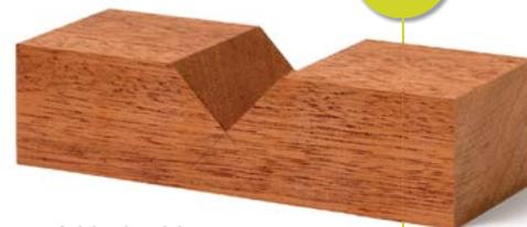
A block with a V-shaped notch helps support square work at a convenient angle for breaking edges.
