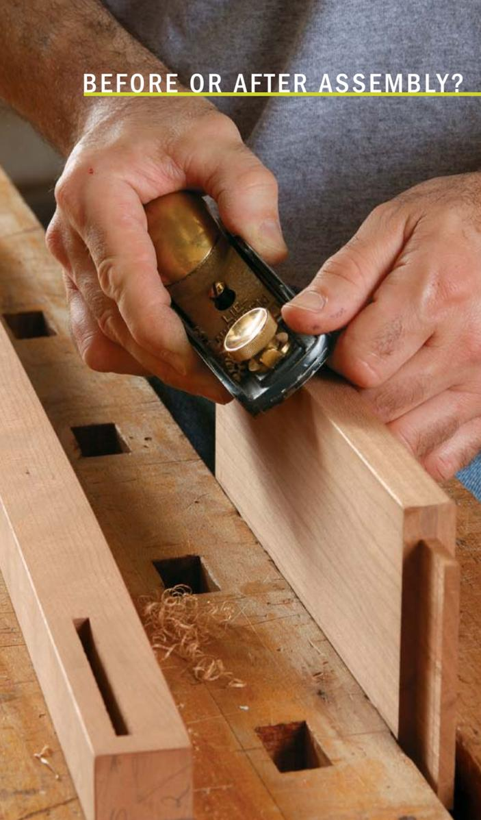
Most edges are easiest to access and work before assembly, but some must wait. Also, be sure to complete surface preparation before breaking edges, as sanding and smoothing can erode the chamfers you've created.
