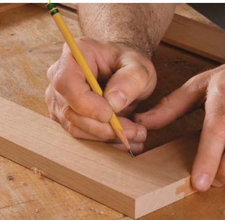
**Mark the stiles.** With the frame dry-fitted, mark the stile at the point where the mating rail will meet it.
