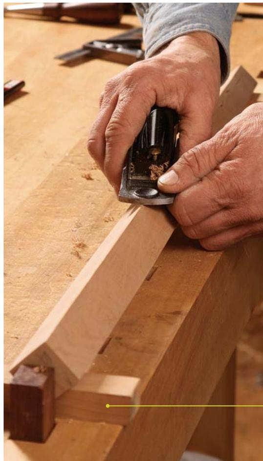
**For long chamfers, guide the plane with both hands. Align the plane's body roughly lengthwise with the corner you're chamfering. Ride a knuckle on the stock to help steady the plane at a consistent angle.**
