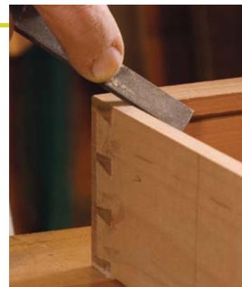
**Out of sight but not out of hand.** Hack uses a gentle roundover on parts like drawer sides that will be handled but not often seen (left). He supports the paper with thick leather. Use a common mill file to get into tight corners (above), skewing it as you push it along the edge.
