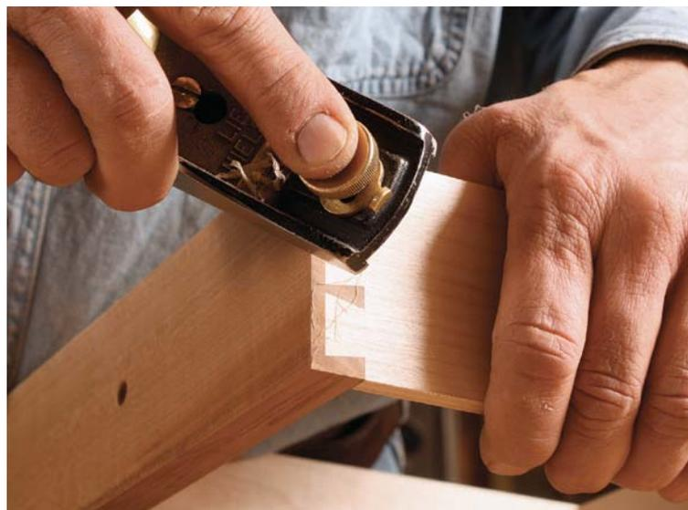
**Get the right angle on end grain. Skewing the iron to the plane's line of travel lowers the cutting angle and pushes the fibers downward, creating a cleaner chamfer at the end of a piece.**
