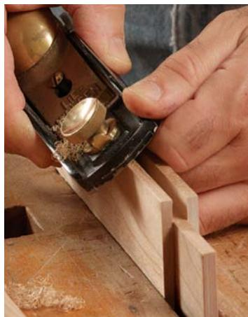
**The rails are easier.** Because the rails die into the adjoining stiles, the chamfers can continue to the end of the workpiece.
