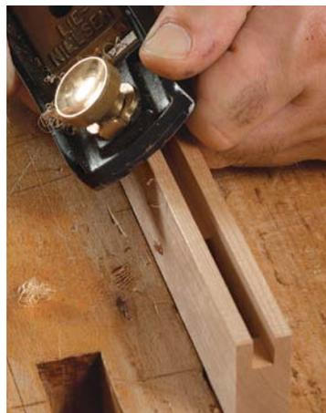
**Don't go too far.** If the chamfer on the stile goes beyond your reference line, it will create a gap in the joint with the rail.
