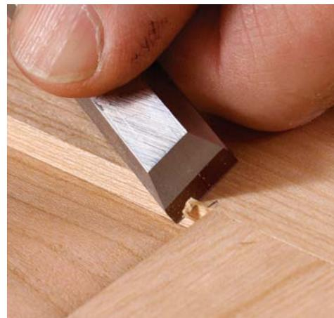
**Finish after assembly.** Use a chisel to carry the chamfer into the corner on the inside of the stile.
