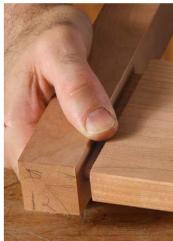
**Advance work.** The bottom edges of a table apron are easily chamfered before glue-up (left), as are the table's legs. Assemble the leg and apron after cutting the chamfers. Cutting these chamfers after assembly would be next to impossible because the adjoining parts obstruct the work (above).
