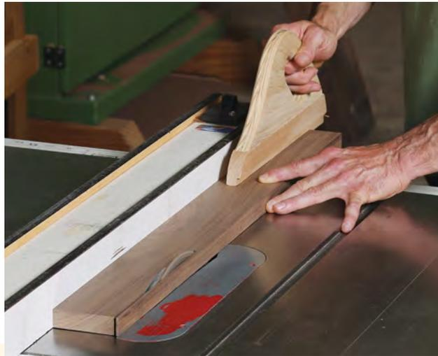
**Two-handed technique.** Your left hand, anchored near the edge of the table, applies downward pressure and keeps the workpiece against the fence. Push the workpiece through the blade with your right hand (above). To keep your right hand well clear of the blade, start using a push stick when your hand reaches the table (left).
