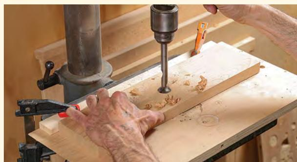
**Two ways to prevent spinning work.** A clamp with a deep throat applies stabilizing pressure right next to the bit (left), and keeps the workpiece from spinning or lifting from the table as you back out the bit. A fence clamped to the drill-press table prevents it from spinning as well (above).
