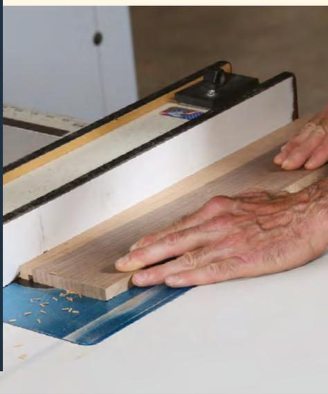
**Two hands, one fence, plenty of control.** No downward pressure is needed, but use your left hand to press the workpiece against the fence. Once again, your right hand feeds it through the cut, counteracting the force of the bit.
