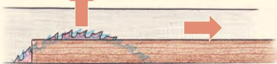
If the feed pressure is not in line with the force exerted by the blade, another force comes into play, causing the workpiece to pivot away from the fence.
