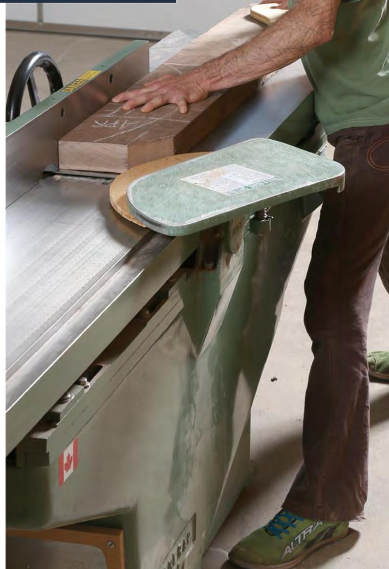
**Press down and push.** Use your left hand to keep the board flat on the jointer's table while pushing it forward with your right hand.
