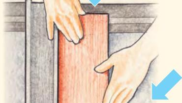
Apply downward and lateral pressure with off hand.
