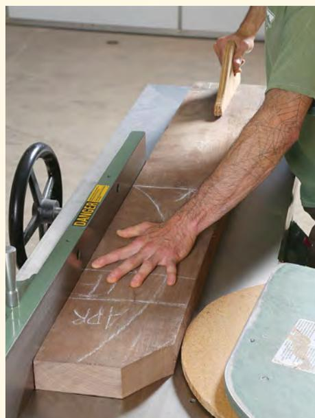
**Keep pressure near the cutterhead.** After the board is 6 in. to 12 in. past the cutterhead, let it pass under your left hand, but continue to apply downward pressure.
